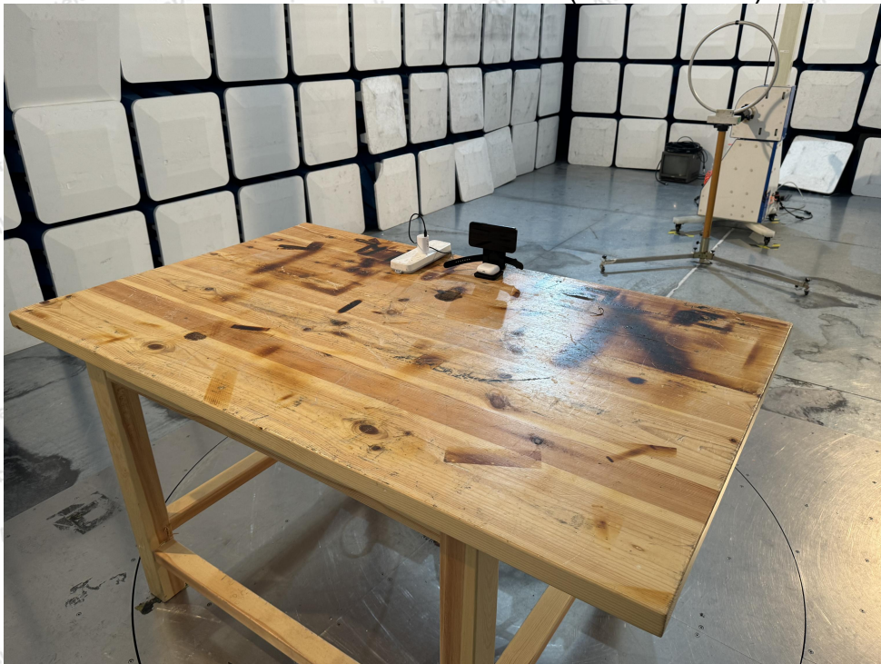
Photo of Radiation Emission Test (below 30MHz)
