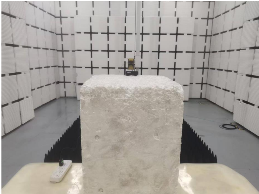
Set-up for Radiated Spurious Emission, Above 1GHz
