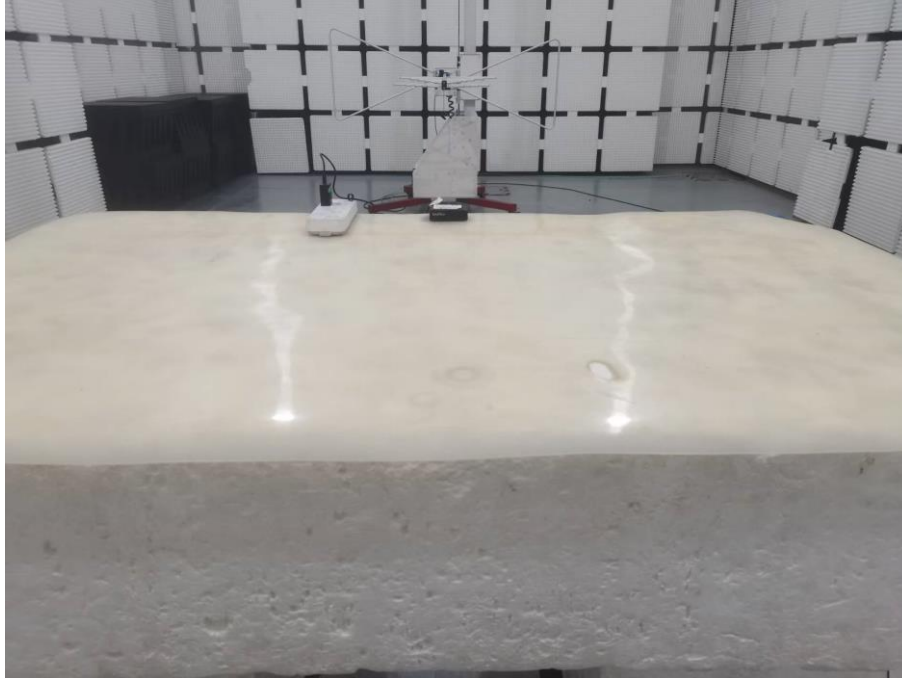
Set-up for Radiated Spurious Emission, Above 1GHz
