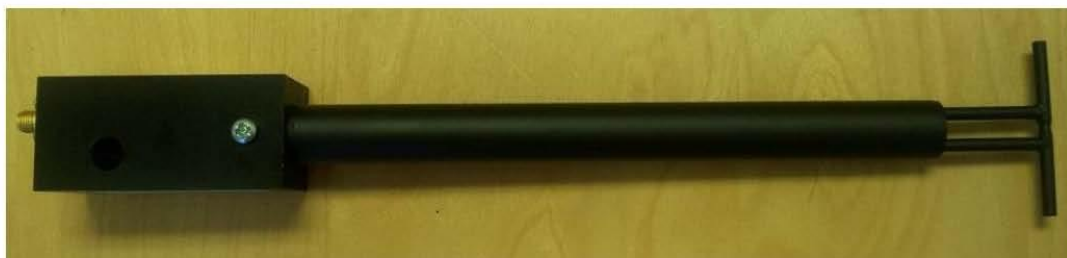
Figure 1 – MVG COMOSAR Validation Dipole
