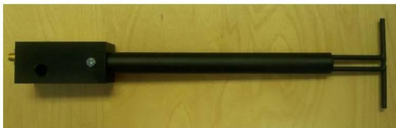
Figure 1 – MVG COMOSAR Validation Dipole
