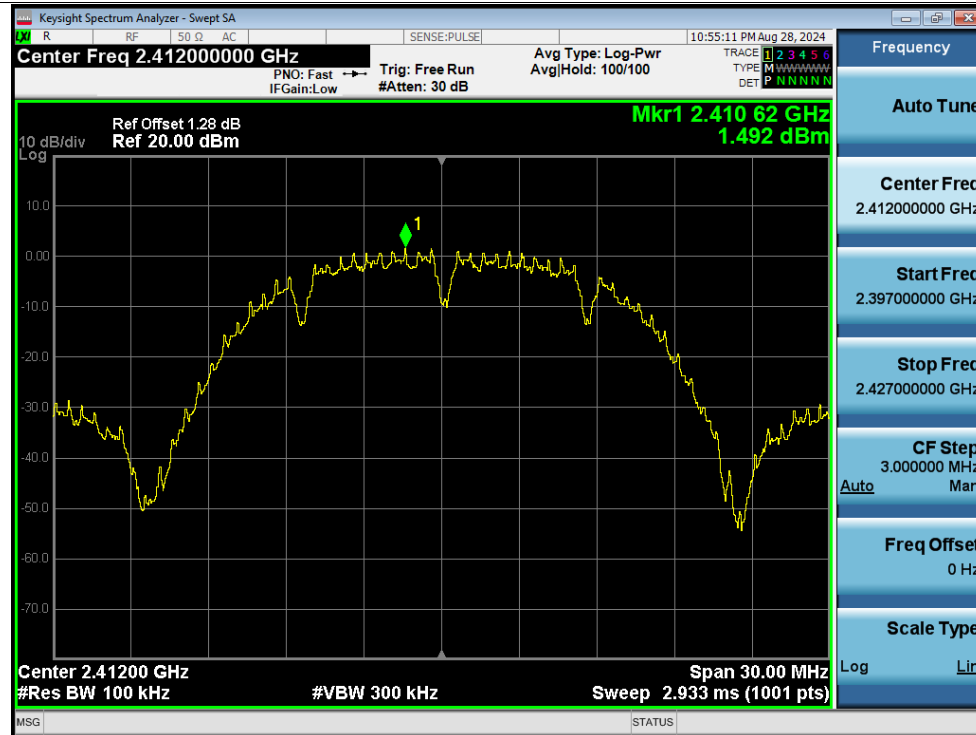
Band Edge NVNT b 2412MHz Ant1 Emission
