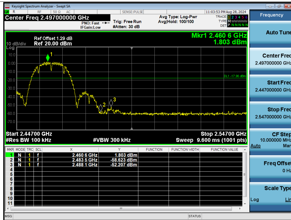
Band Edge NVNT b 2462MHz Ant1 Emission
