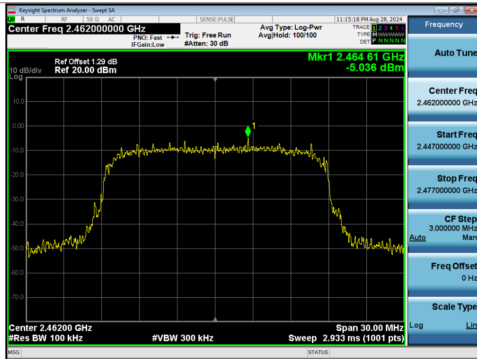
Band Edge NVNT g 2462MHz Ant1 Emission
