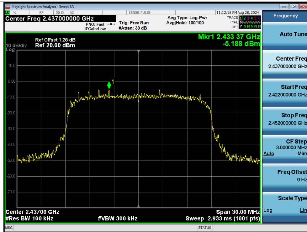
Tx. Spurious NVNT g 2437MHz Ant1 Emission
