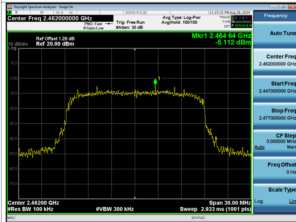
Tx. Spurious NVNT g 2462MHz Ant1 Emission
