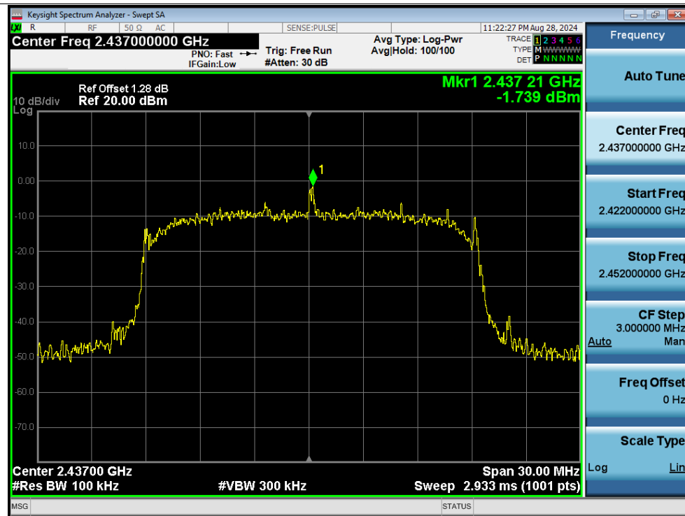
Tx. Spurious NVNT n20 2437MHz Ant1 Emission
