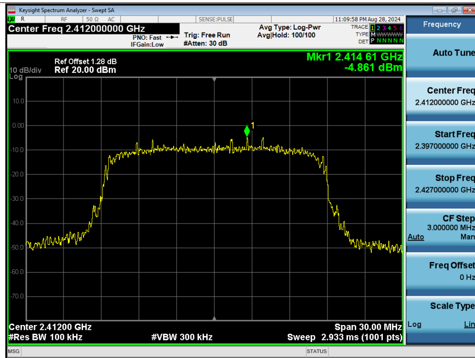
Tx. Spurious NVNT g 2412MHz Ant1 Emission
