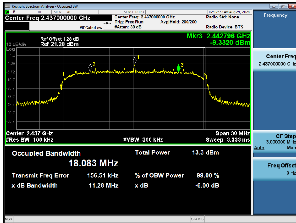
-6dB Bandwidth NVNT n20 2437MHz Ant1
