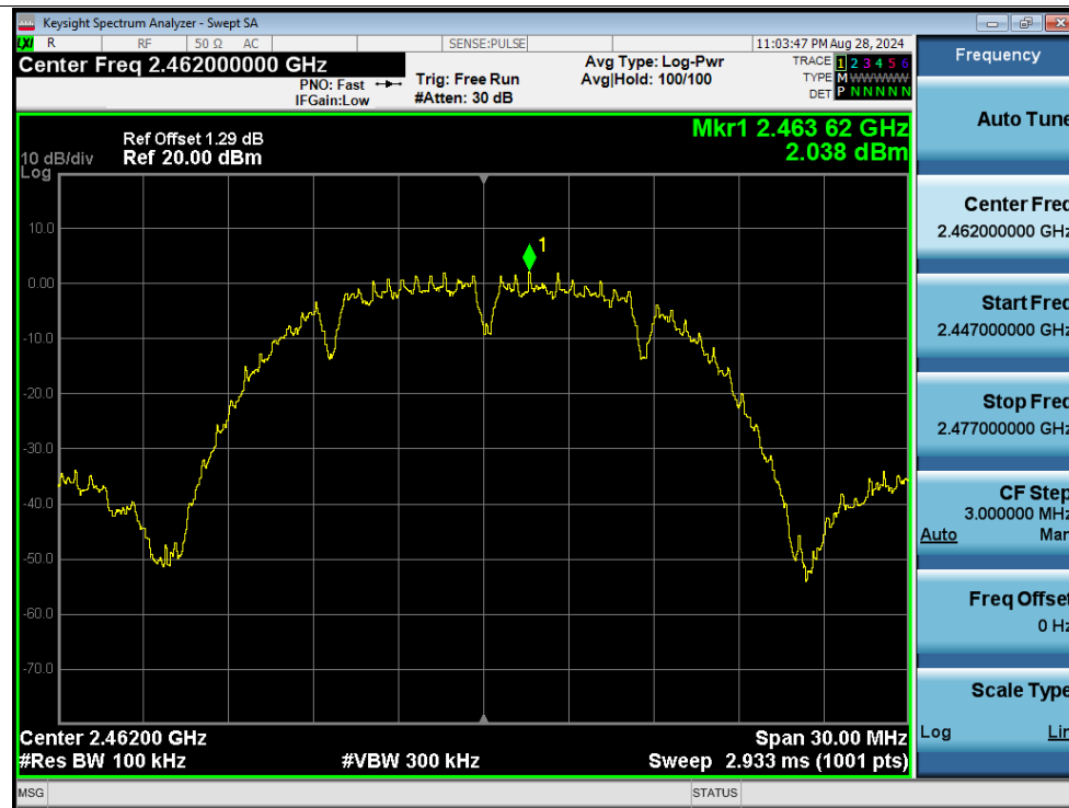
Band Edge NVNT b 2462MHz Ant1 Emission
