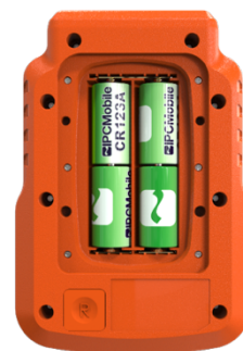
FIGURE 8: The 4 CR123A Batteries are Aligned in 2S-2P Configuration
