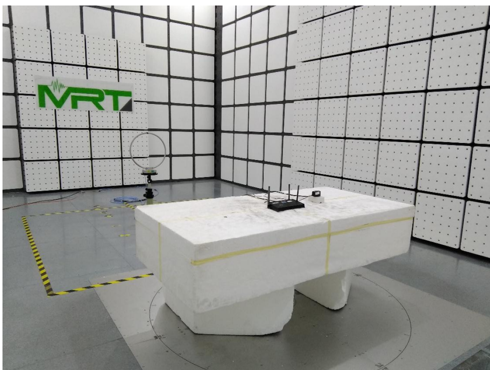
Description: Radiated Emission Test Setup for 9kHz~30MHz
