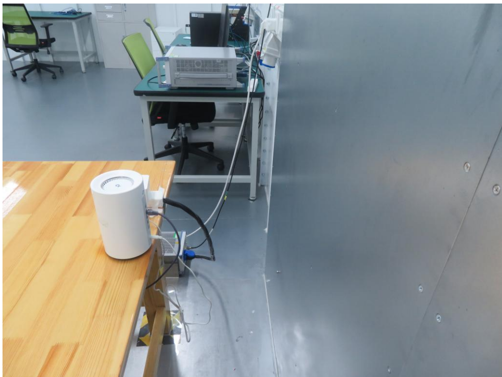
Description: Conducted Emissions Test Setup (WJ-SR5)
