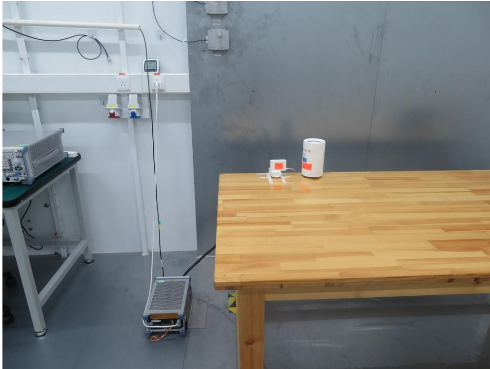
Description: Conducted Emissions Test Setup (WJ-SR5)
