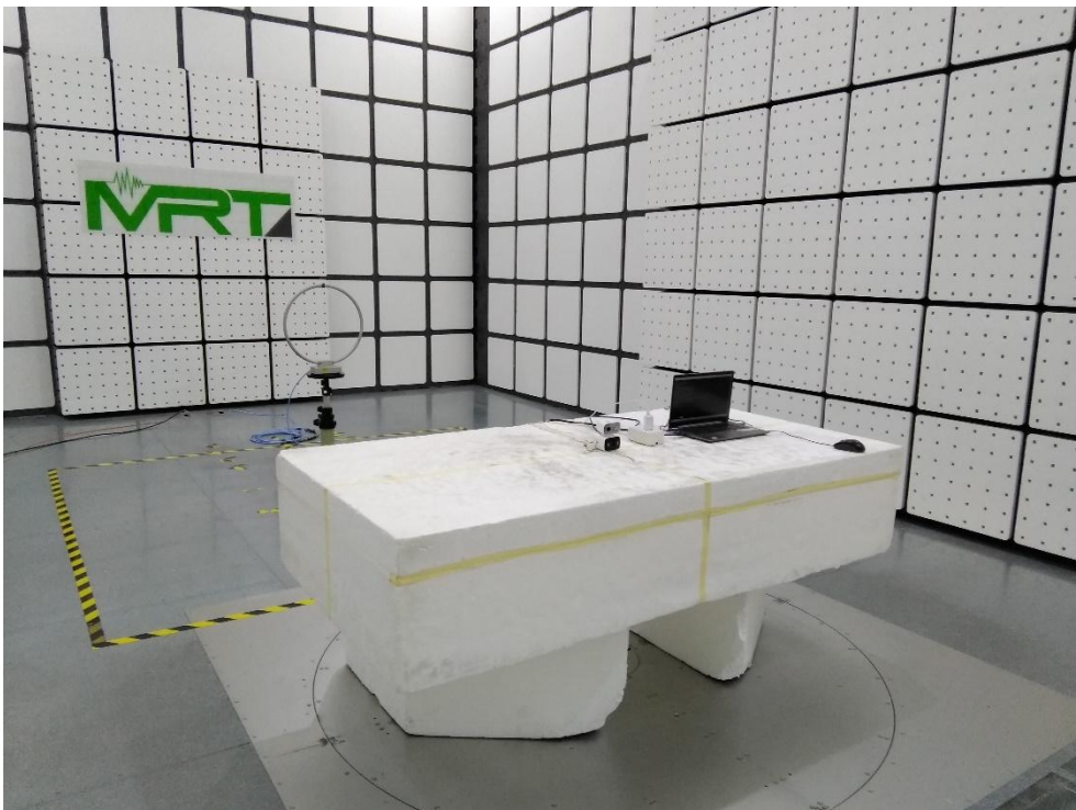
Description: Radiated Emission Test Setup for 9kHz~30MHz
