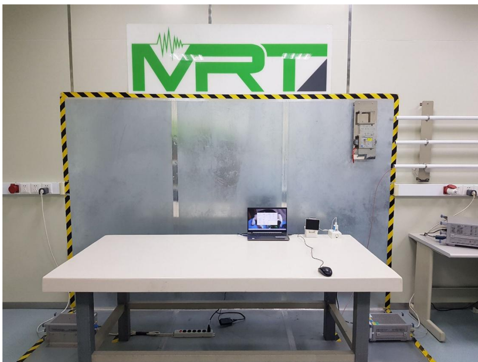
Description: Side View of Conducted Emission Test Setup_WiFi
