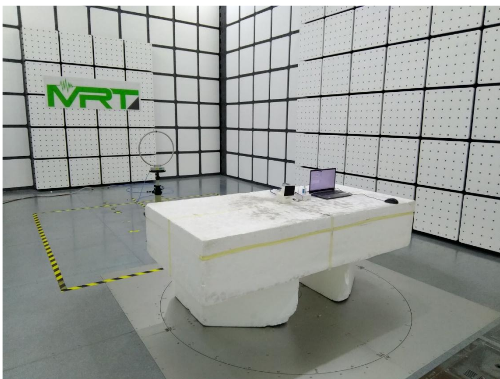
Description: Radiated Emission Test Setup for 9kHz~30MHz_BLE
