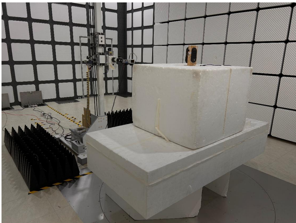
Description: Radiated Emission Test Setup for 9kHz~30MHz (BLE)
