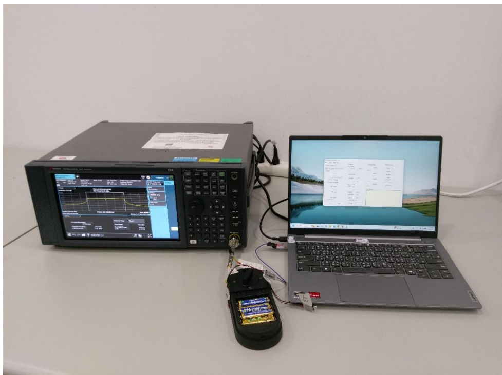
Description: Conducted Measurement Test Setup (WiFi)
