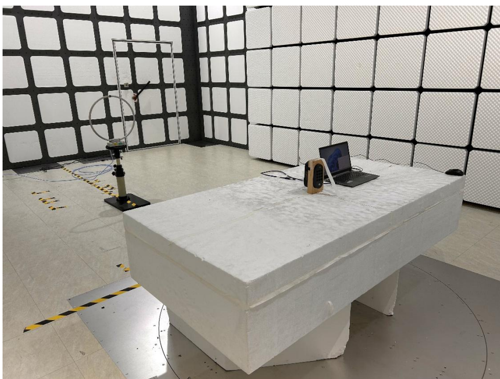
Description: Radiated Emission Test Setup for 9kHz~30MHz (BLE)
