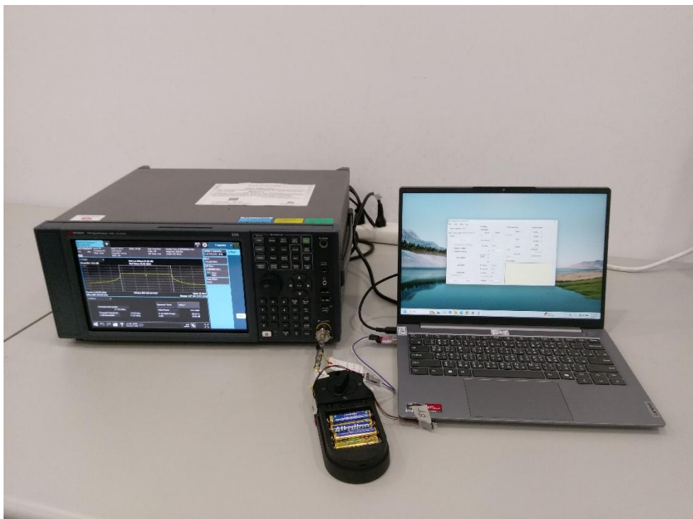
Description: Conducted Measurement Test Setup (WiFi)
