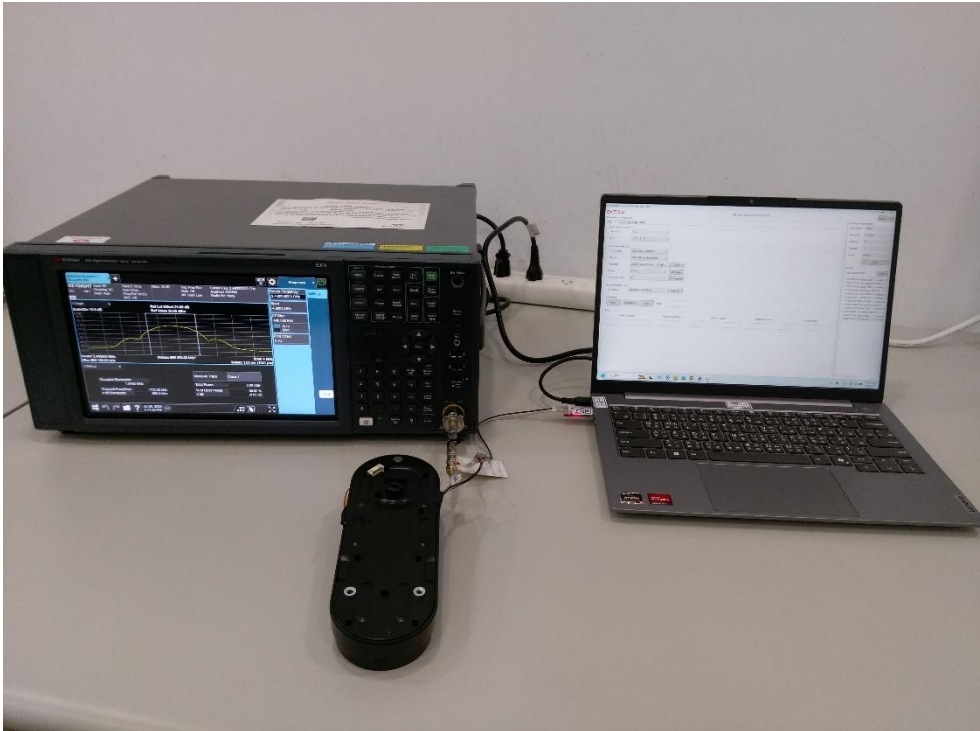
Description: Conducted Measurement Test Setup (WiFi)
