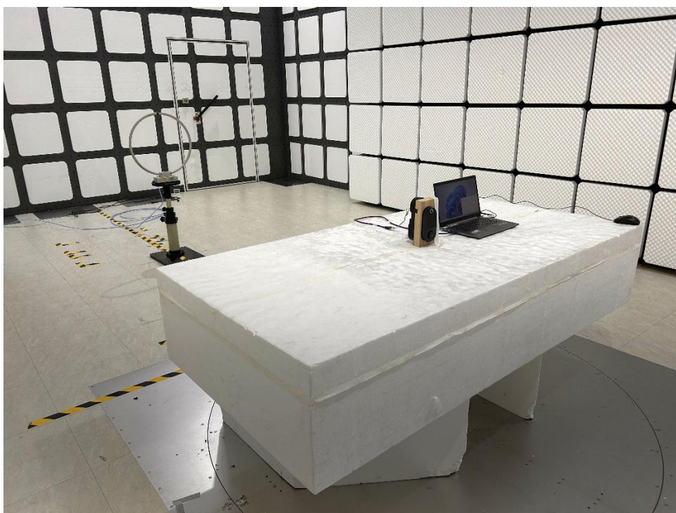
Description: Radiated Emission Test Setup for 9kHz~30MHz (WiFi)
