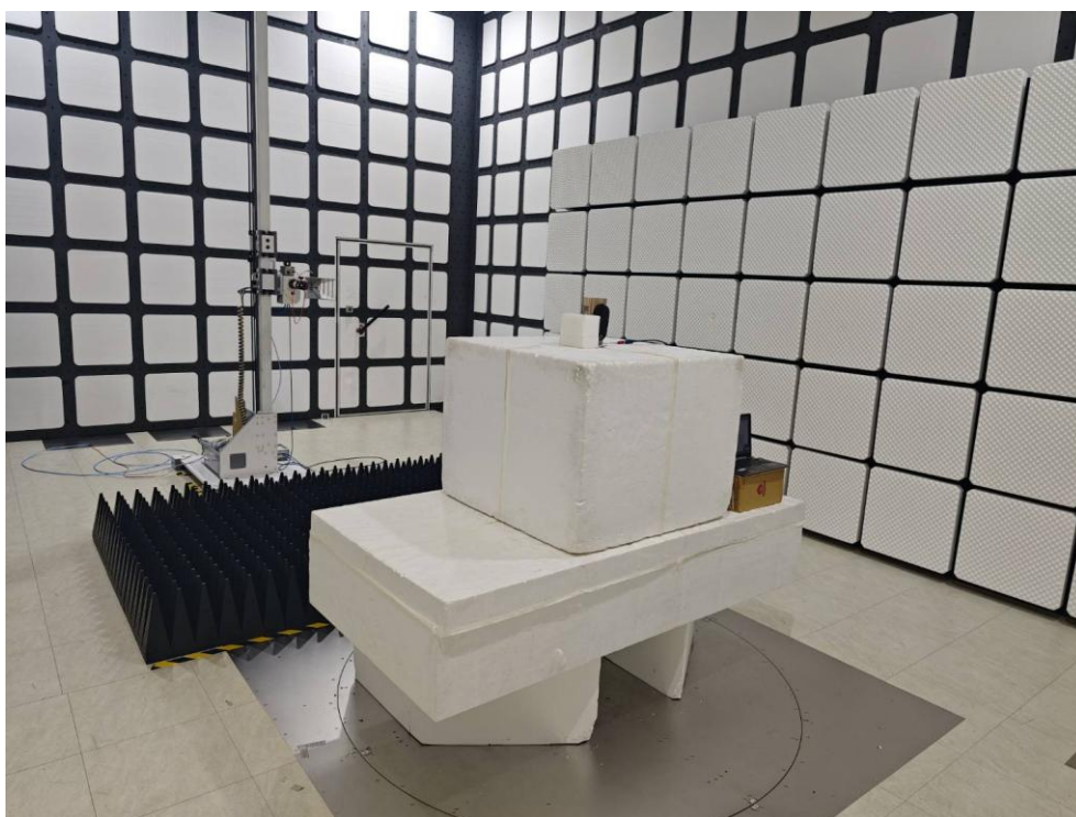
Description: Radiated Emission Test Setup for above 1GHz (WiFi)
