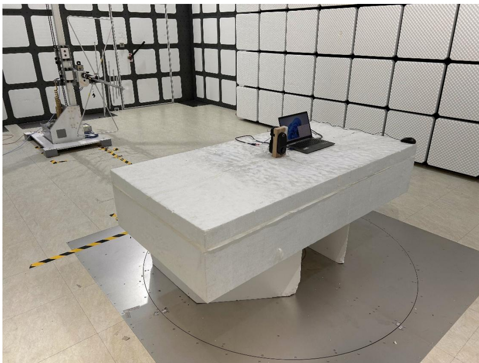
Description: Radiated Emission Test Setup for above 1GHz (WiFi)
