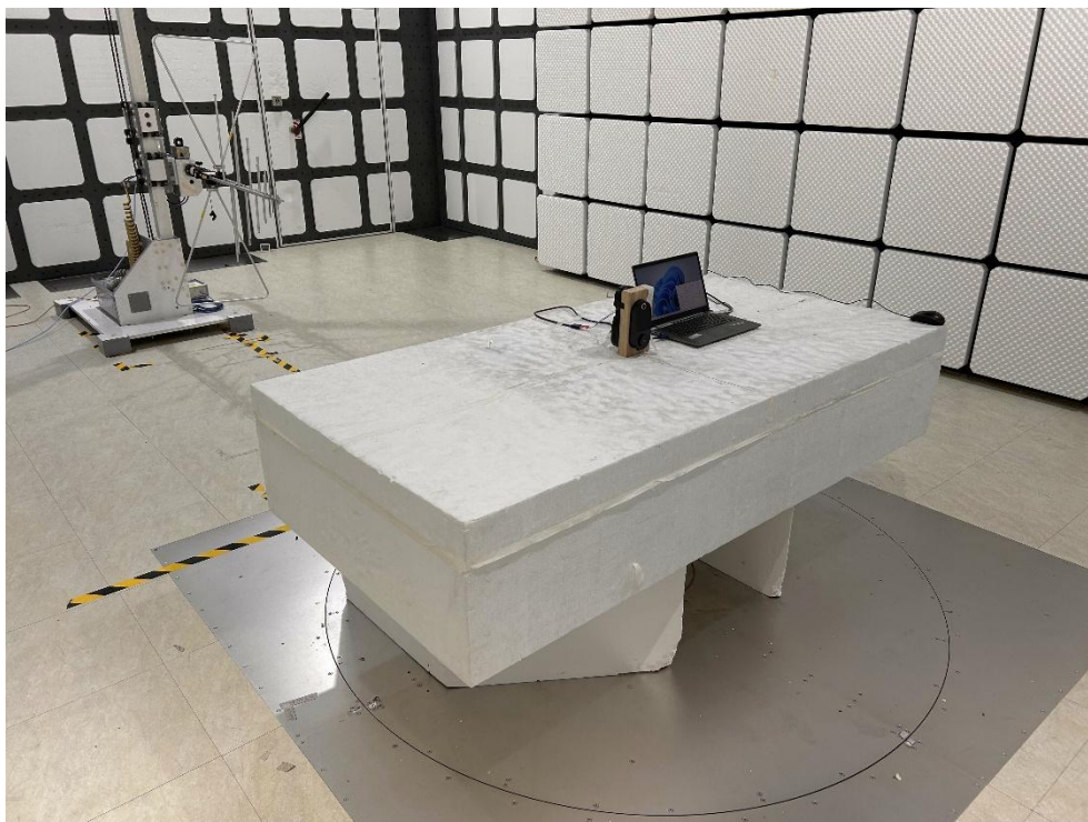
Description: Radiated Emission Test Setup for above 1GHz (BLE)
