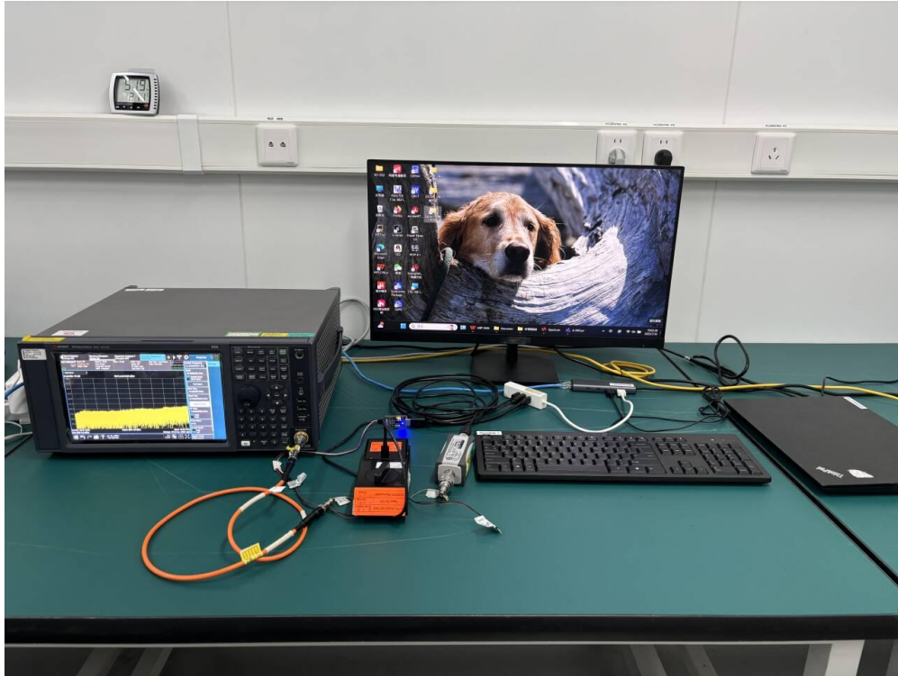
Description: Front View of AC Conducted Emissions Test Setup (WJ-SR5)
