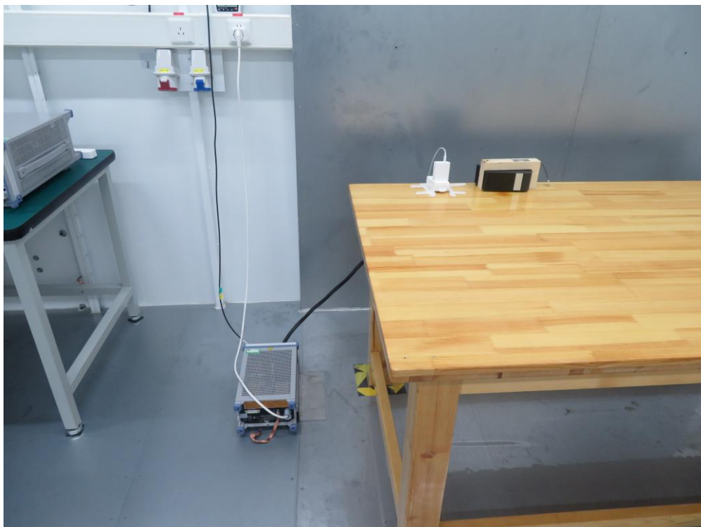
Description: Front View of AC Conducted Emissions Test Setup (WJ-SR5)
