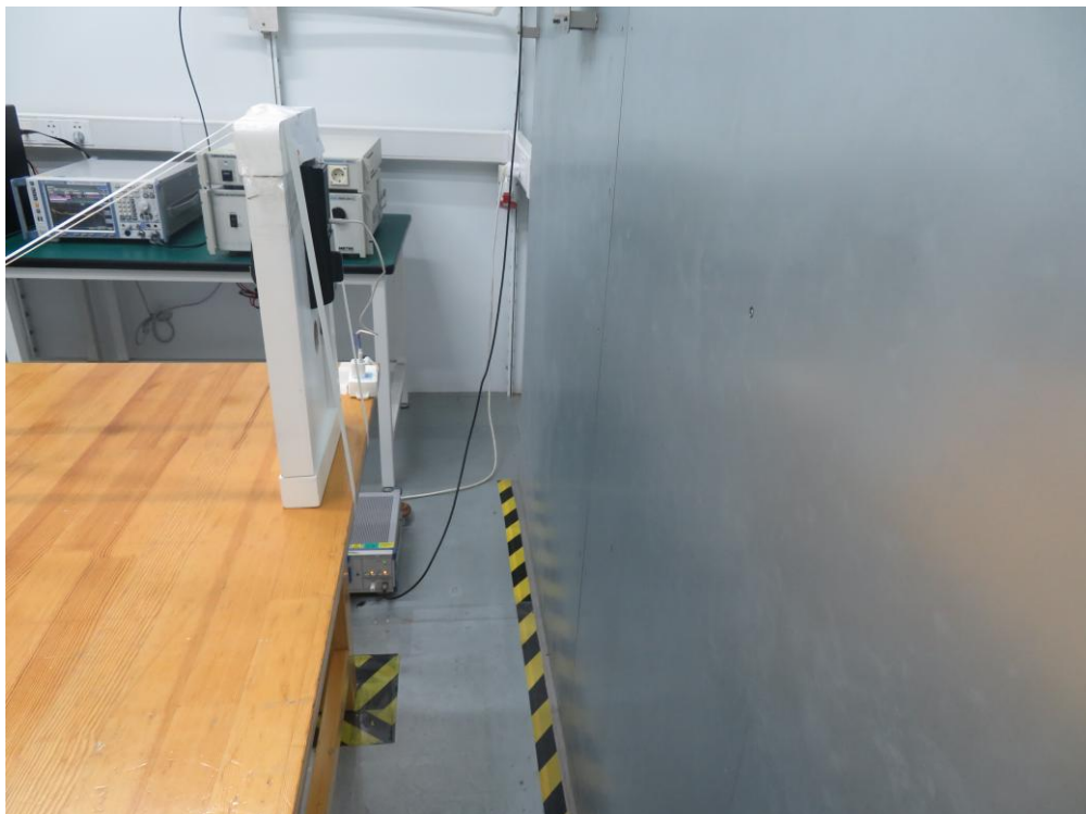
Description: Side View of AC Conducted Emissions Test Setup (SIP-SR2)
