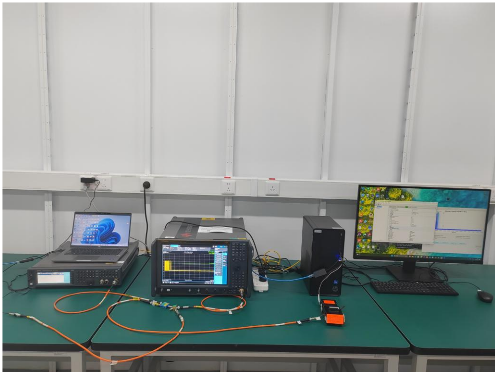
Description: Dynamic Frequency Selection Test Setup (WJ-SR7)
