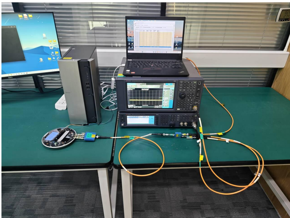
Description: Dynamic Frequency Selection Test Setup
