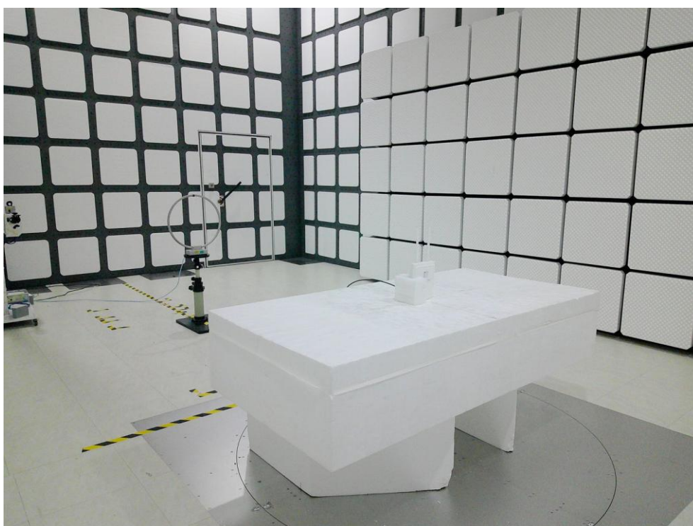
Description: Radiated Emission Test Setup for 9kHz~30MHz
