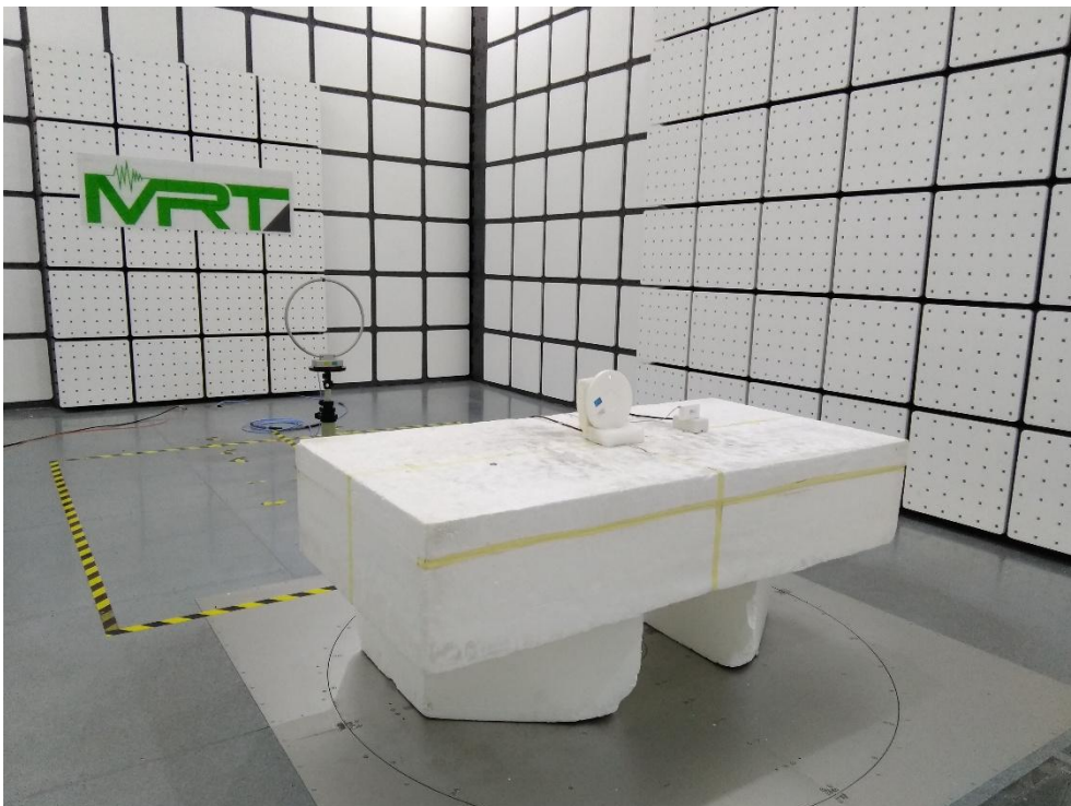
Description: Radiated Emission Test Setup for 9kHz~30MHz
