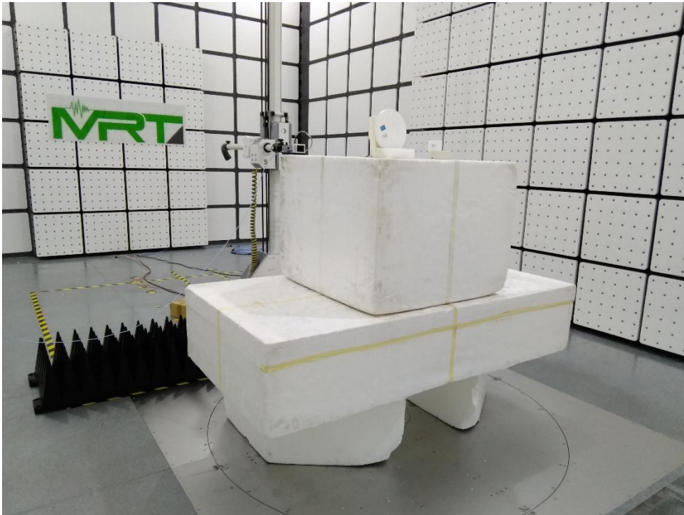
Description: Radiated Emission Test Setup for 9kHz~30MHz
