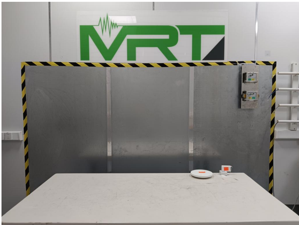
Description: Front View of AC Conducted Emissions Test Setup
