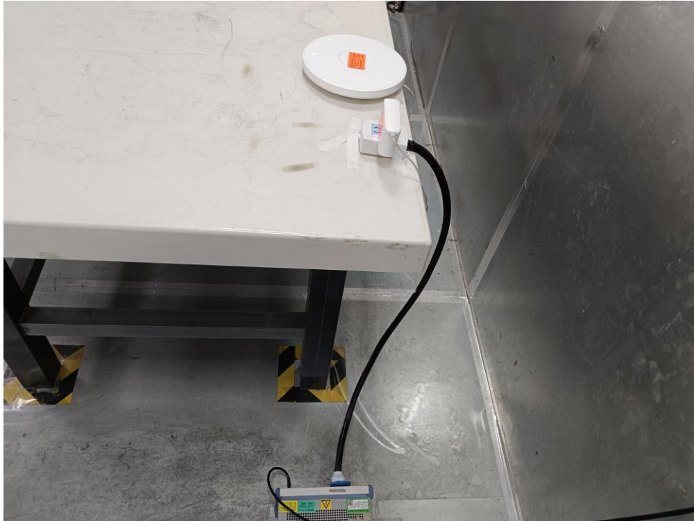
Description: Side View of AC Conducted Emissions Test Setup
