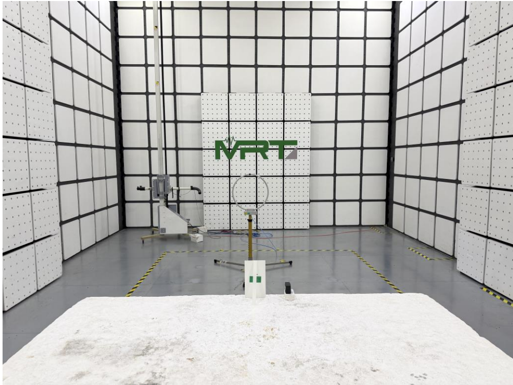
Description: Radiated Spurious Emissions Test Setup for Below 1 GHz
