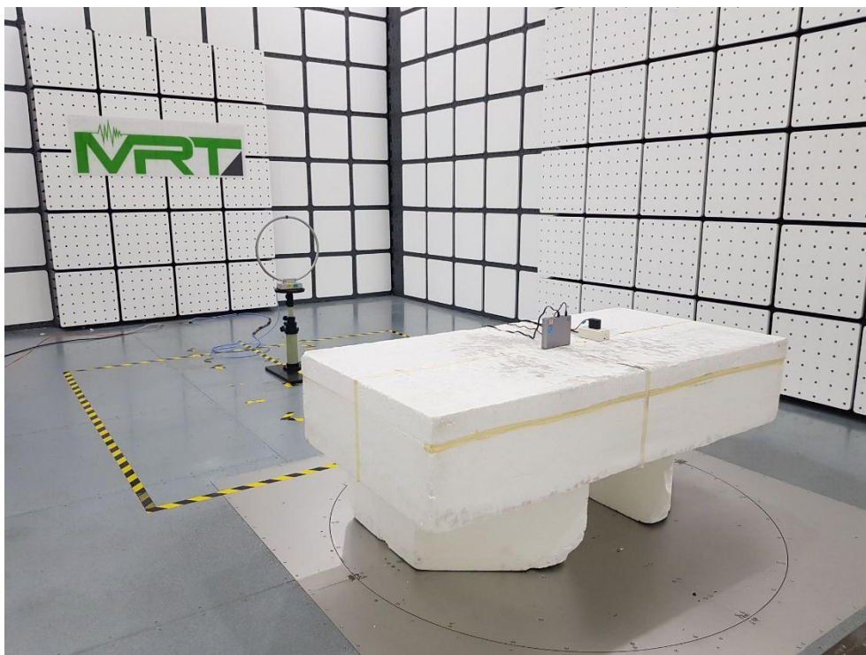
Description: Radiated Emission Test Setup for 9kHz~30MHz
