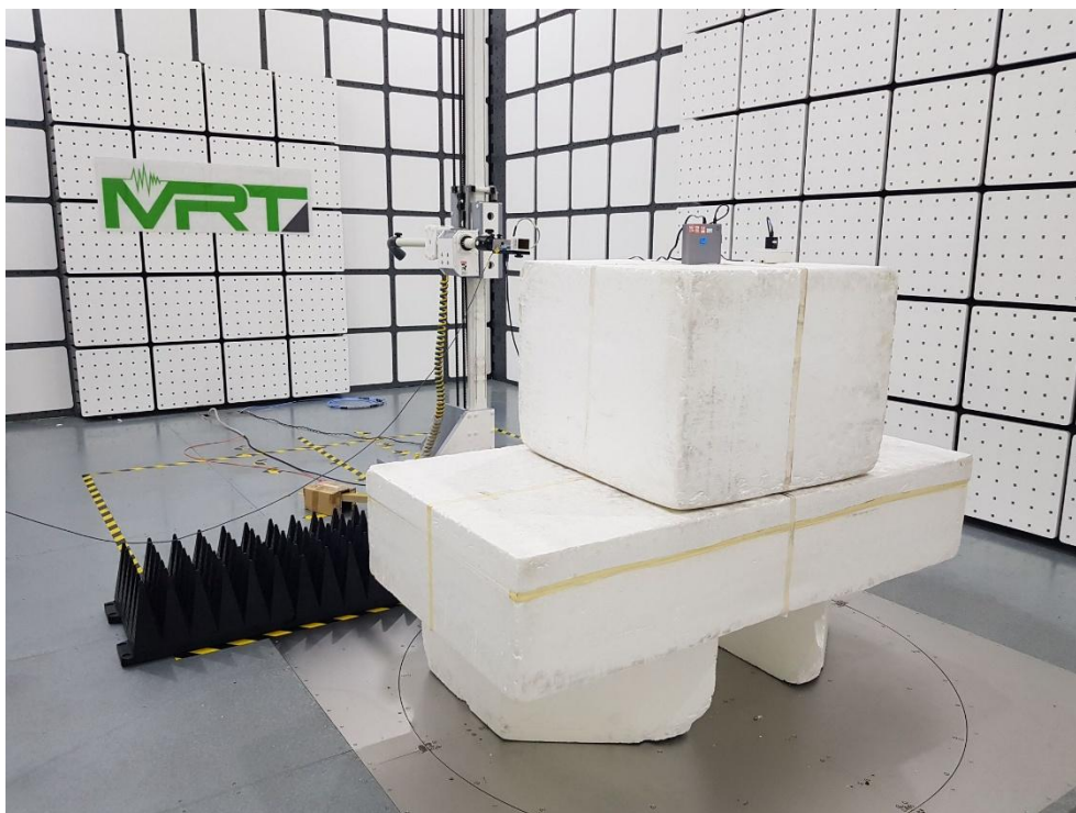
Description: Radiated Emission Test Setup for 9kHz~30MHz
