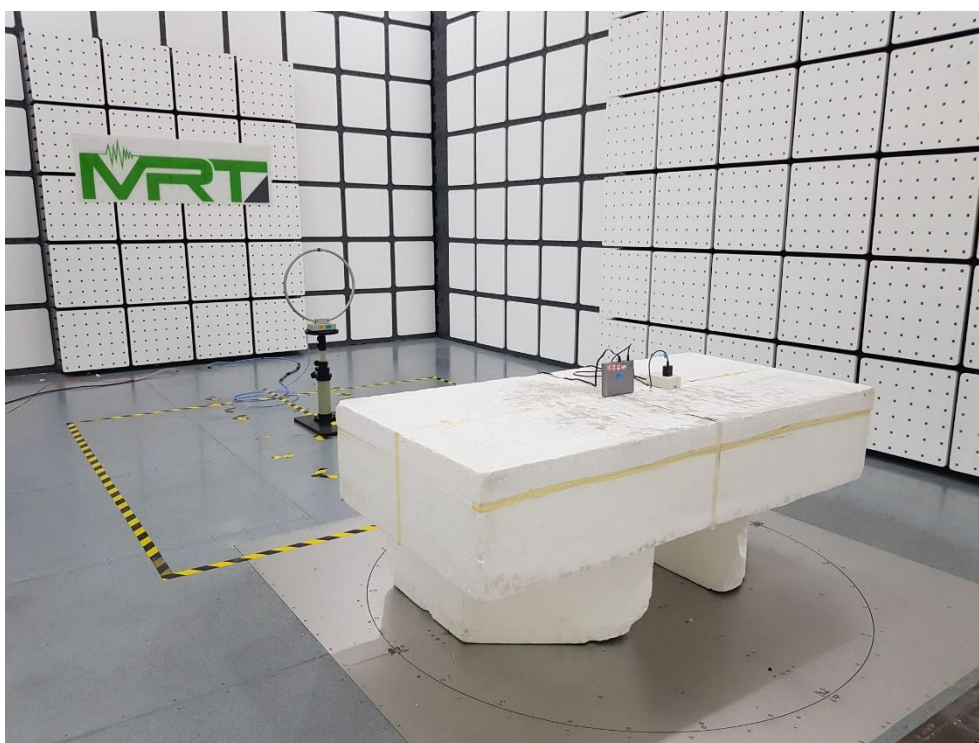
Description: Radiated Emission Test Setup for 9kHz~30MHz
