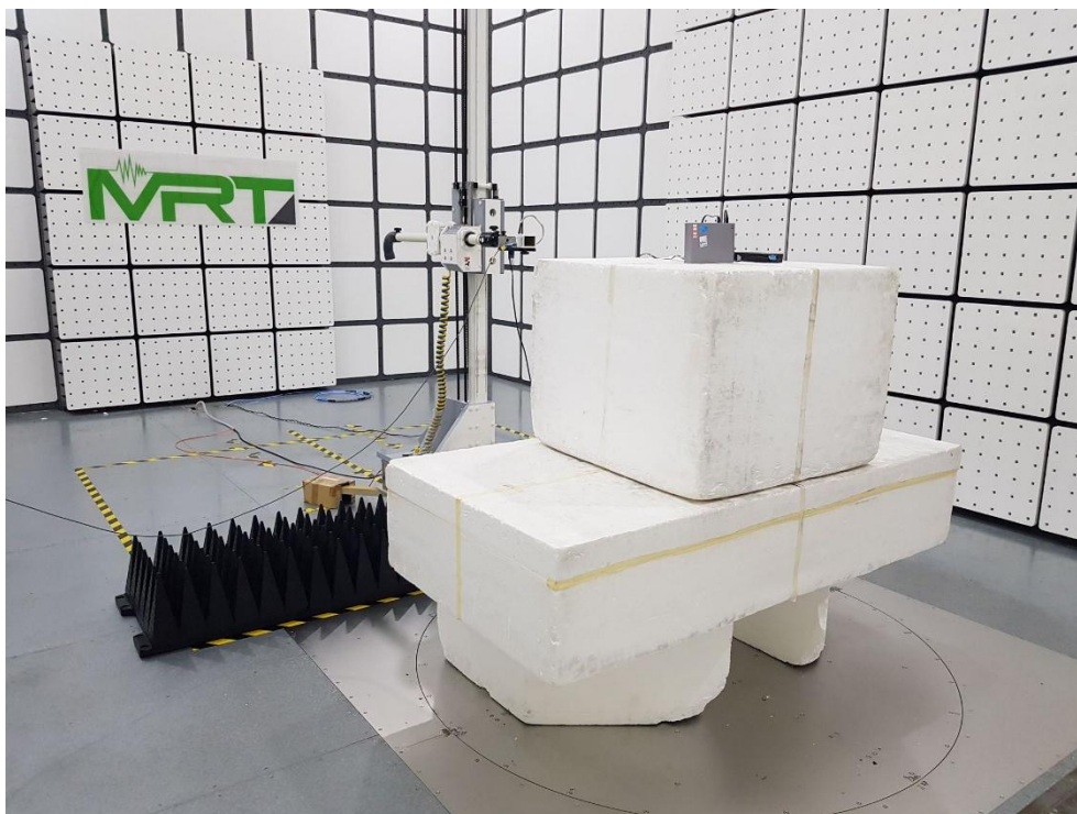
Description: Radiated Emission Test Setup for 9kHz~30MHz
