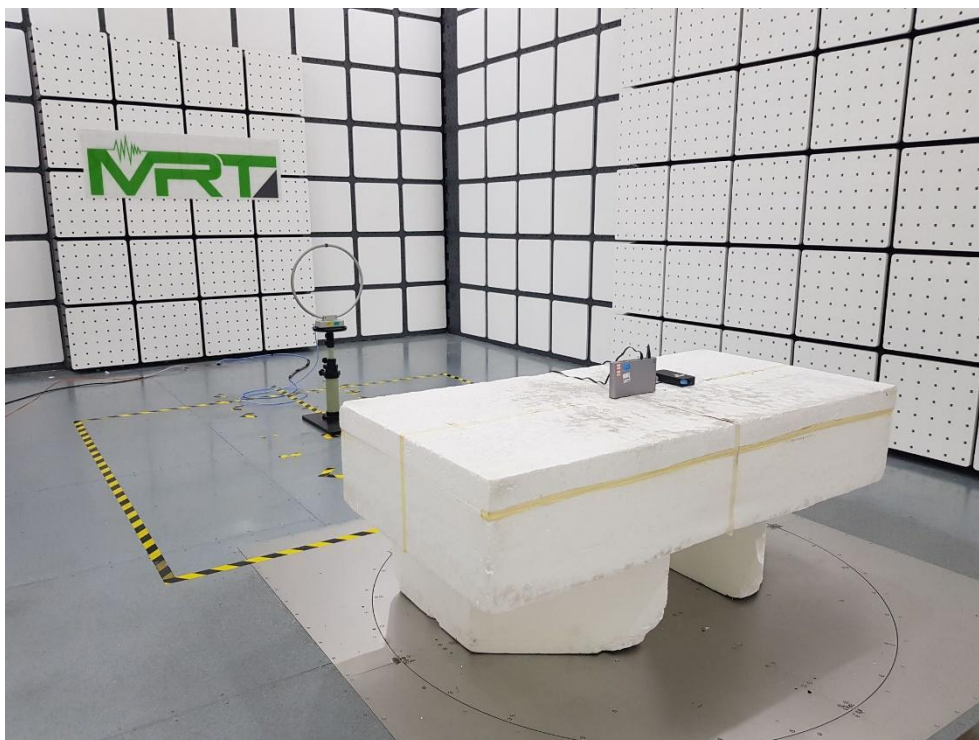
Description: Radiated Emission Test Setup for 9kHz~30MHz
