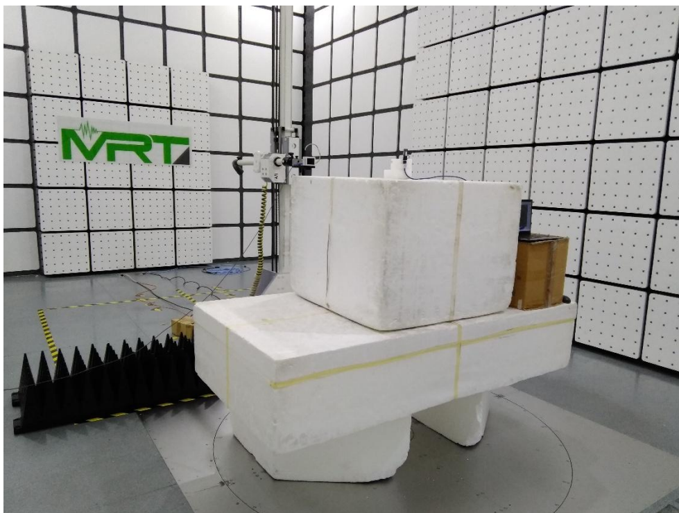
Description: Radiated Emission Test Setup for 9kHz~30MHz
