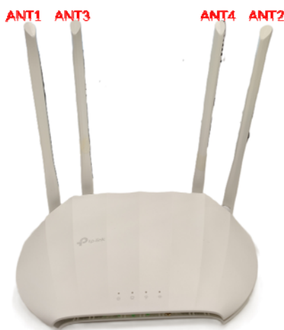
Figure 1-1 Locations of Antennas
