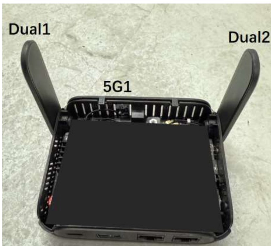
Figure 1-1 Locations of Antennas
