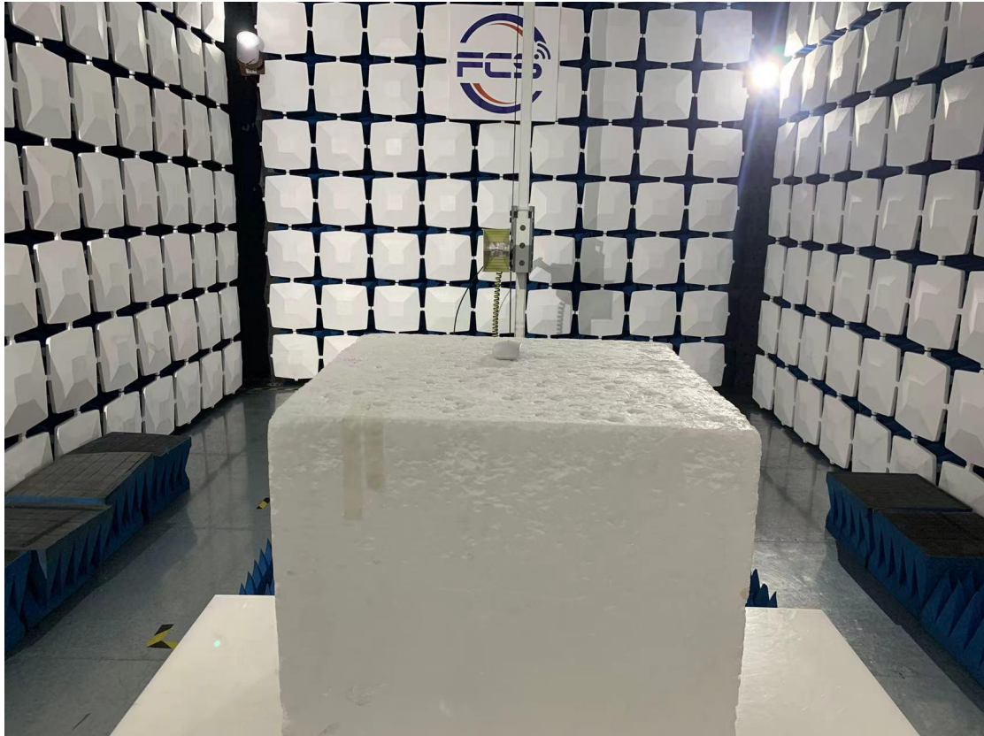
Above 1GHz for radiated emission test setup
