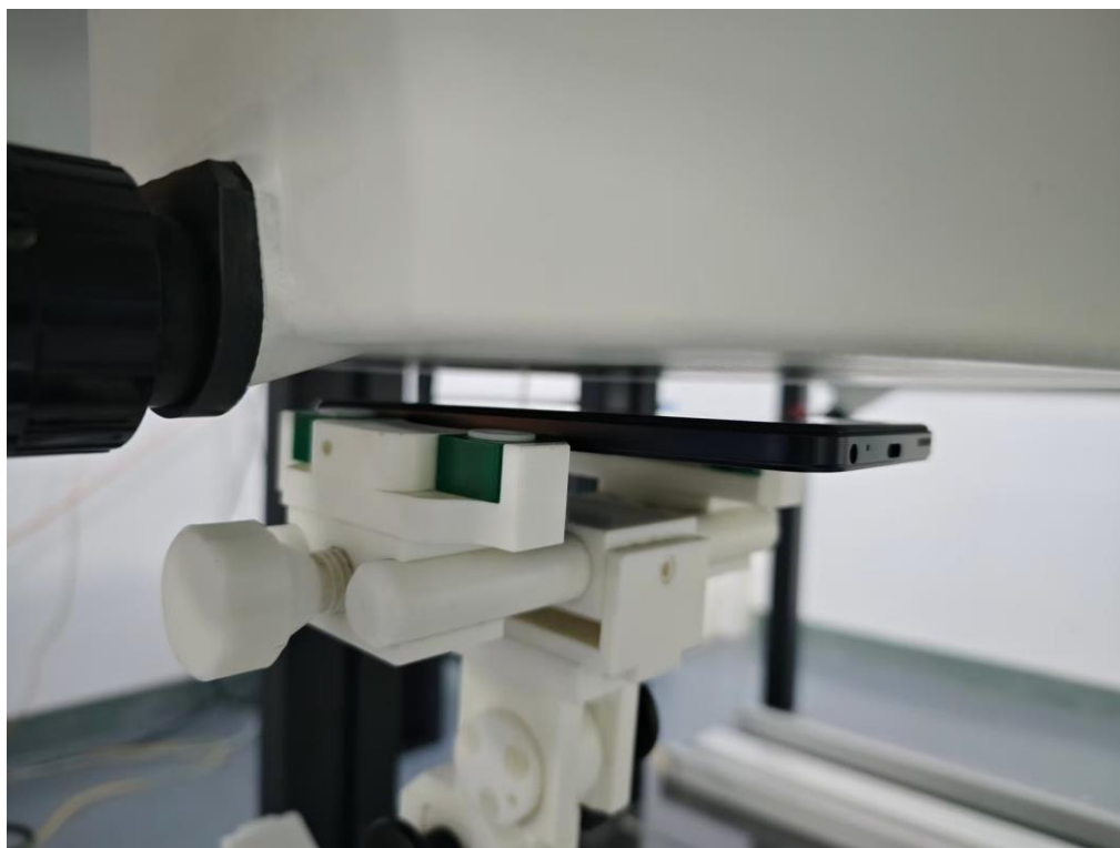
Hotspot Front side (separation distance is 10mm)
