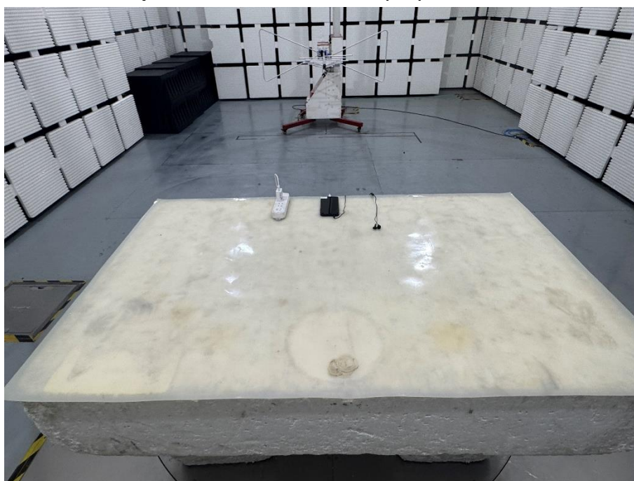
Set-up for Radiated Emission (RE), Below 1GHz
