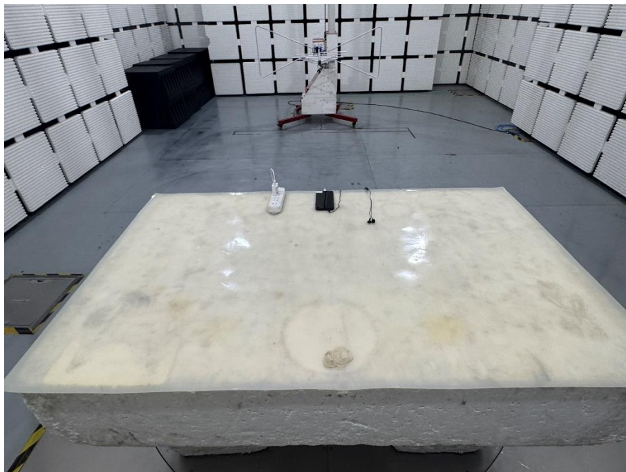
Set-up for Radiated Emission (RE), Below 1GHz
