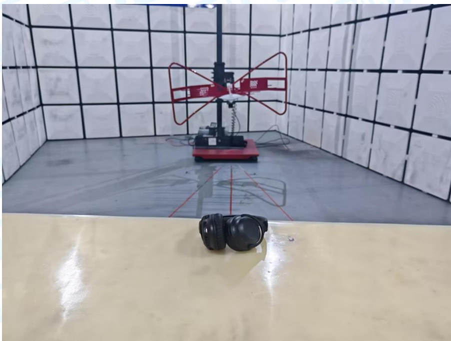
Photo of Setup for Radiated Emission (30MHz~1GHz)
