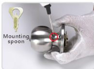
2.Align the hole with the mounting key Push the shrapnel down
