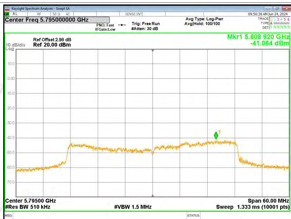
PSD NVNT ac40 5795MHz Ant1
