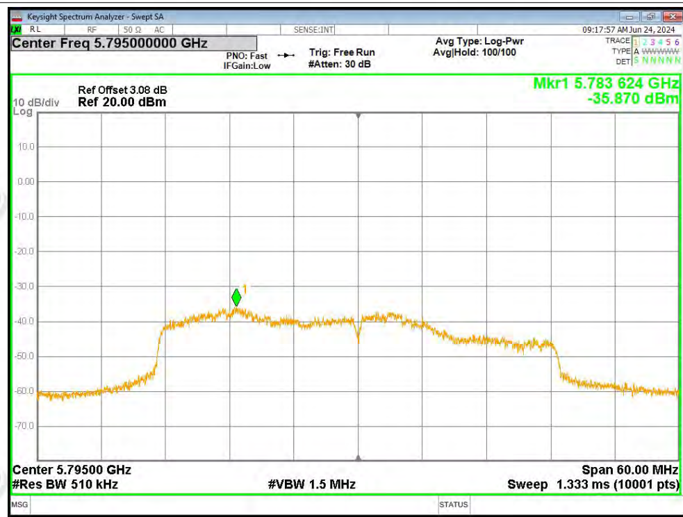
PSD NVNT n40 5795MHz Ant2
