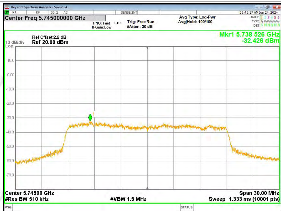
PSD NVNT ac20 5785MHz Ant1
