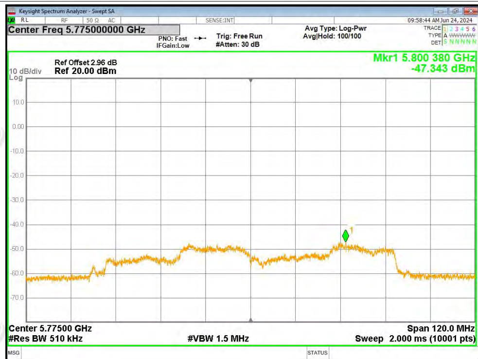
PSD NVNT ac80 5775MHz Ant2
