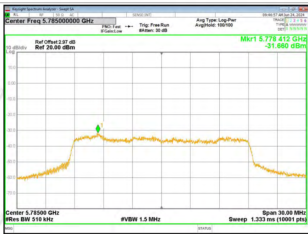
PSD NVNT ac20 5785MHz Ant1
