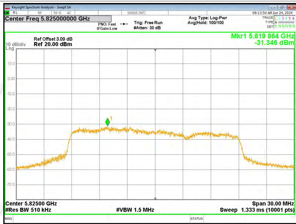
PSD NVNT ac20 5825MHz Ant2
