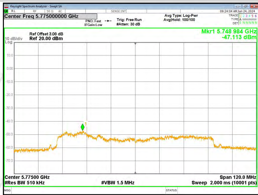
PSD NVNT ac80 5775MHz Ant2
