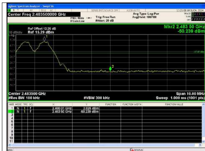
Out Of Band Emission(Right) GFSK_DH5_Channel Hopping
