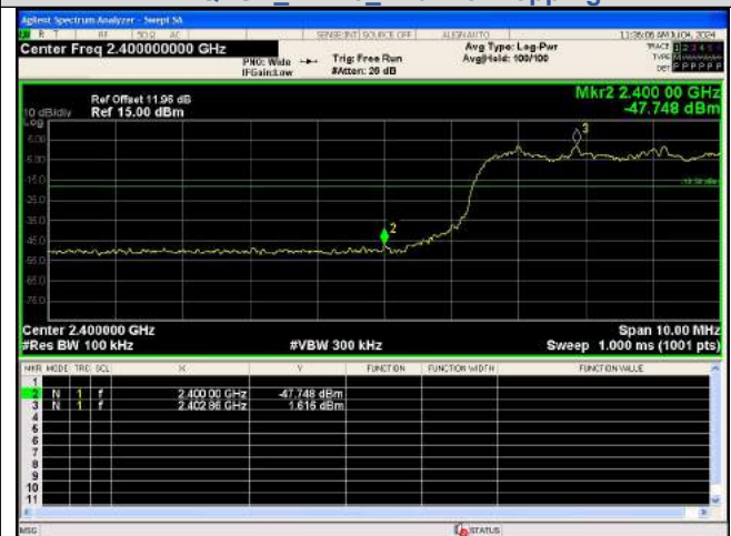
Out Of Band Emission(Left) \pi/4 DQPSK_2-DH5_Channel Hopping
