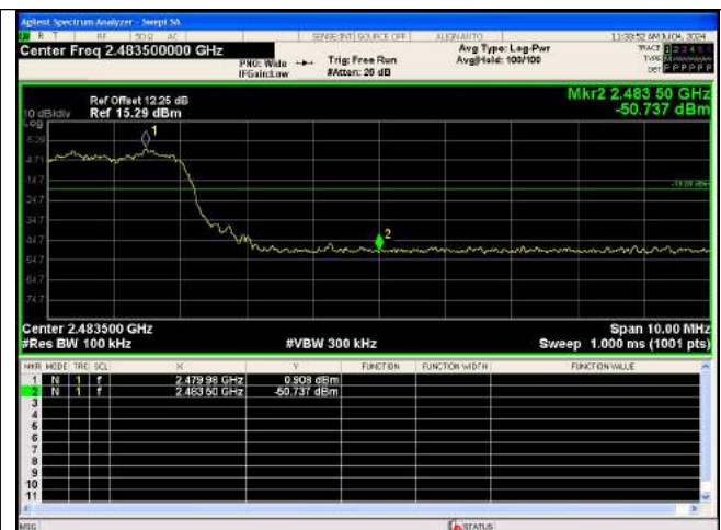
Out Of Band Emission(Right) \pi/4 DQPSK_2-DH5_Channel Hopping
