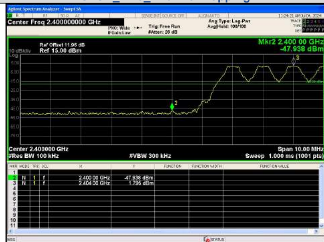
Out Of Band Emission(Left) GFSK_DH5_Channel Hopping
