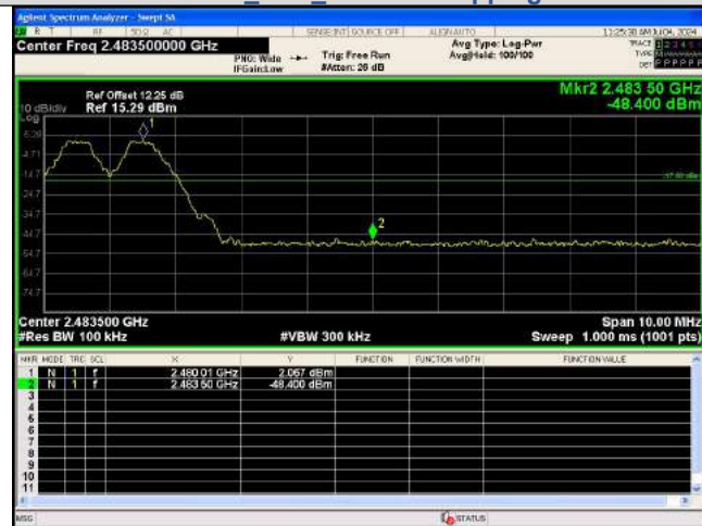
Out Of Band Emission(Right) GFSK_DH5_Channel Hopping
