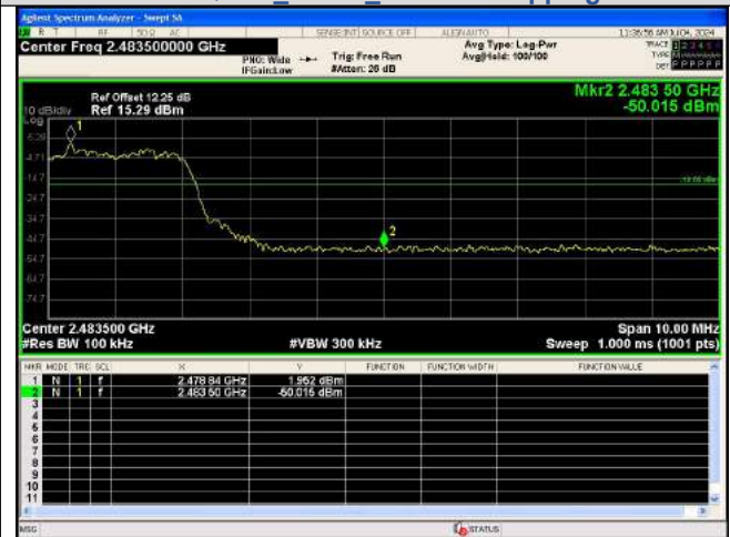
Out Of Band Emission(Right) \pi/4 DQPSK_2-DH5_Channel Hopping
