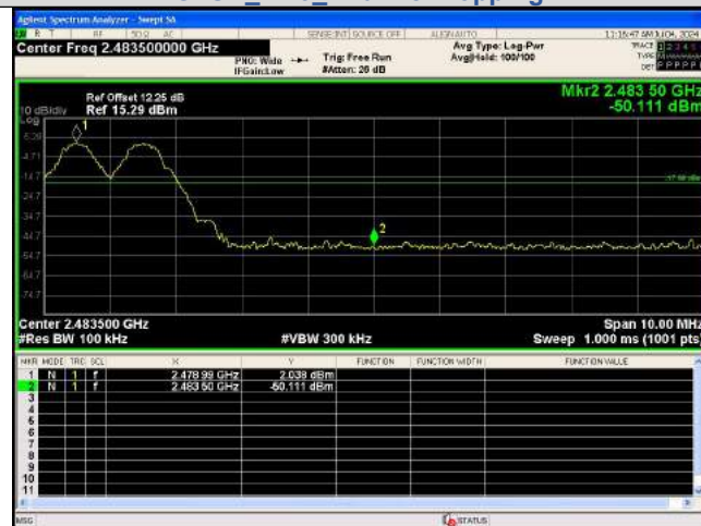
Out Of Band Emission(Right) GFSK_DH5_Channel Hopping
