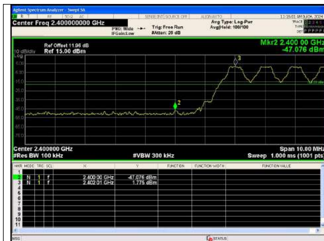
Out Of Band Emission(Left) GFSK_DH5_Channel Hopping
