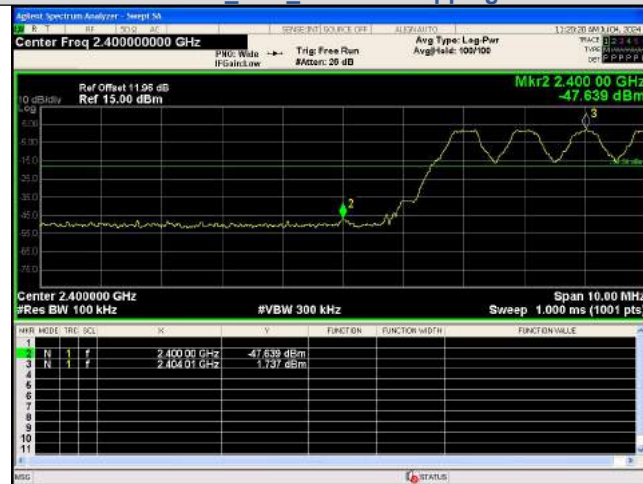
Out Of Band Emission(Left) GFSK_DH5_Channel Hopping
