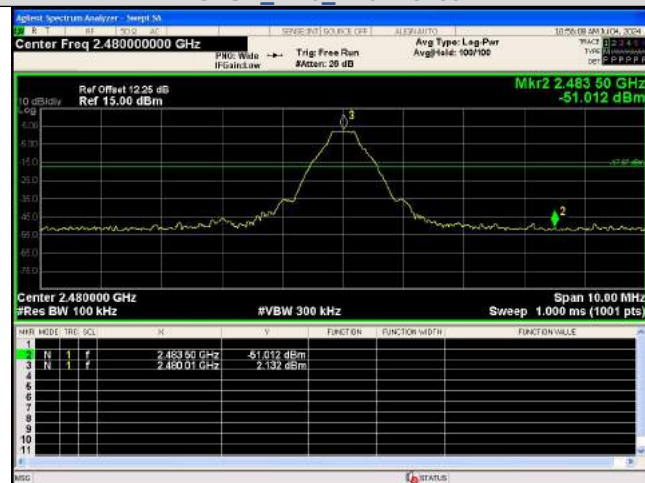
Out Of Band Emission GFSK_DH5_Channel 78
