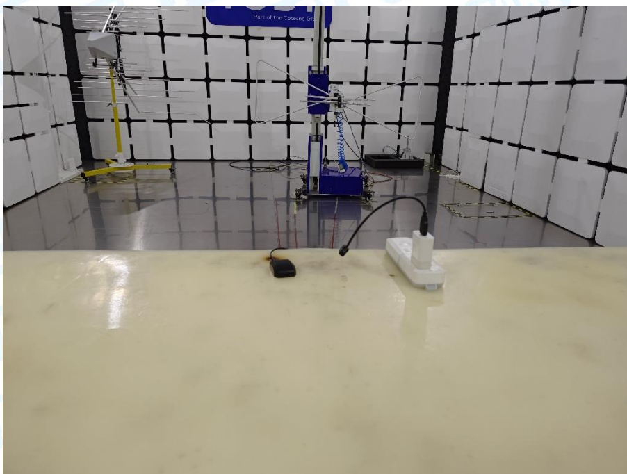
Photo of Setup for Radiated Emission (30MHz~1GHz)
