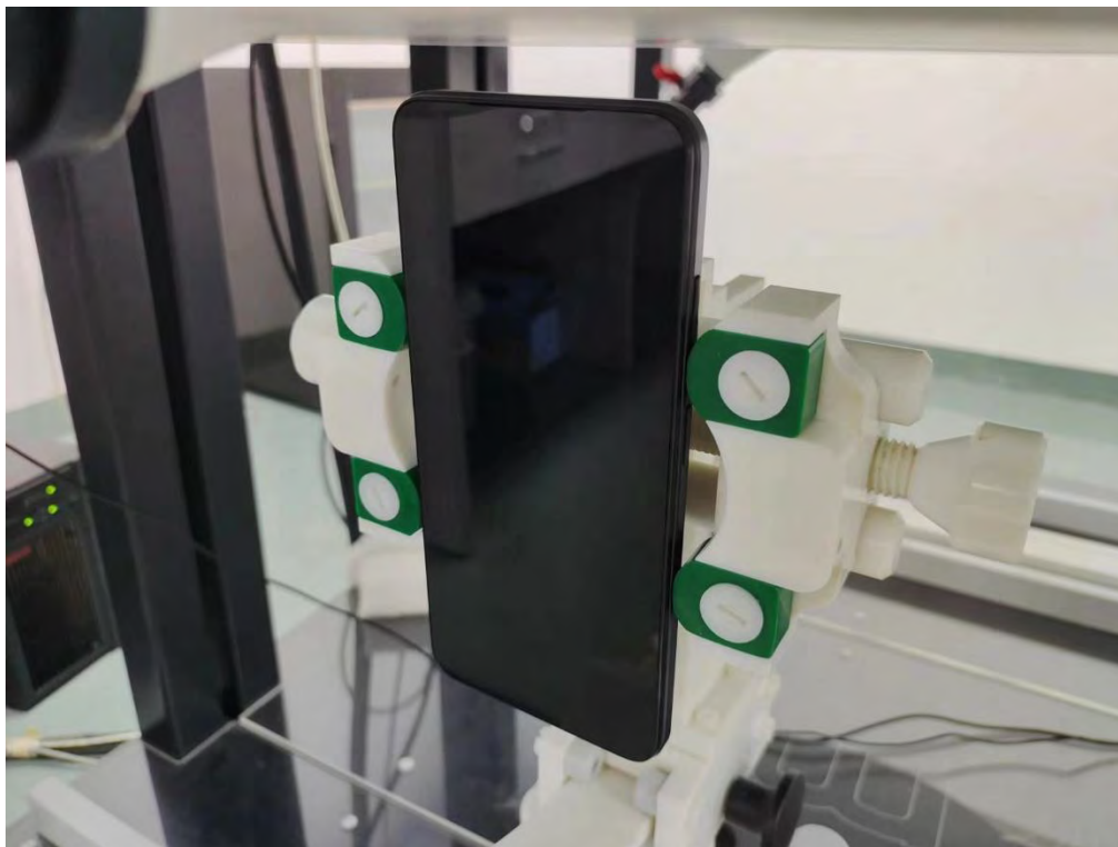
Body Top side (separation distance is 10mm)
