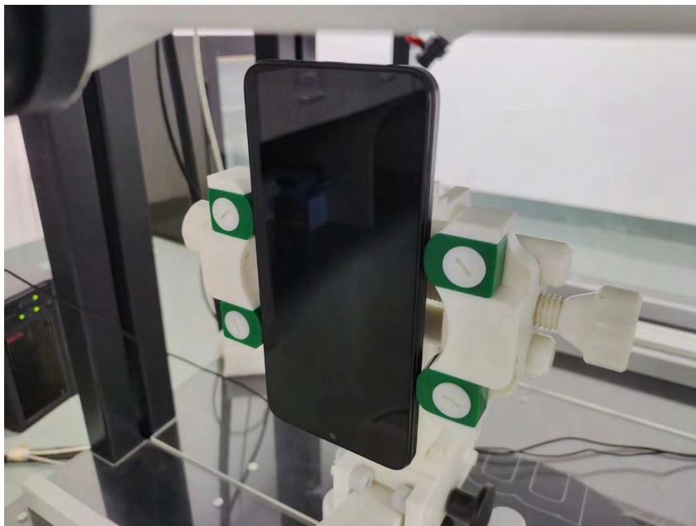
Body Bottom side (separation distance is 10mm)
