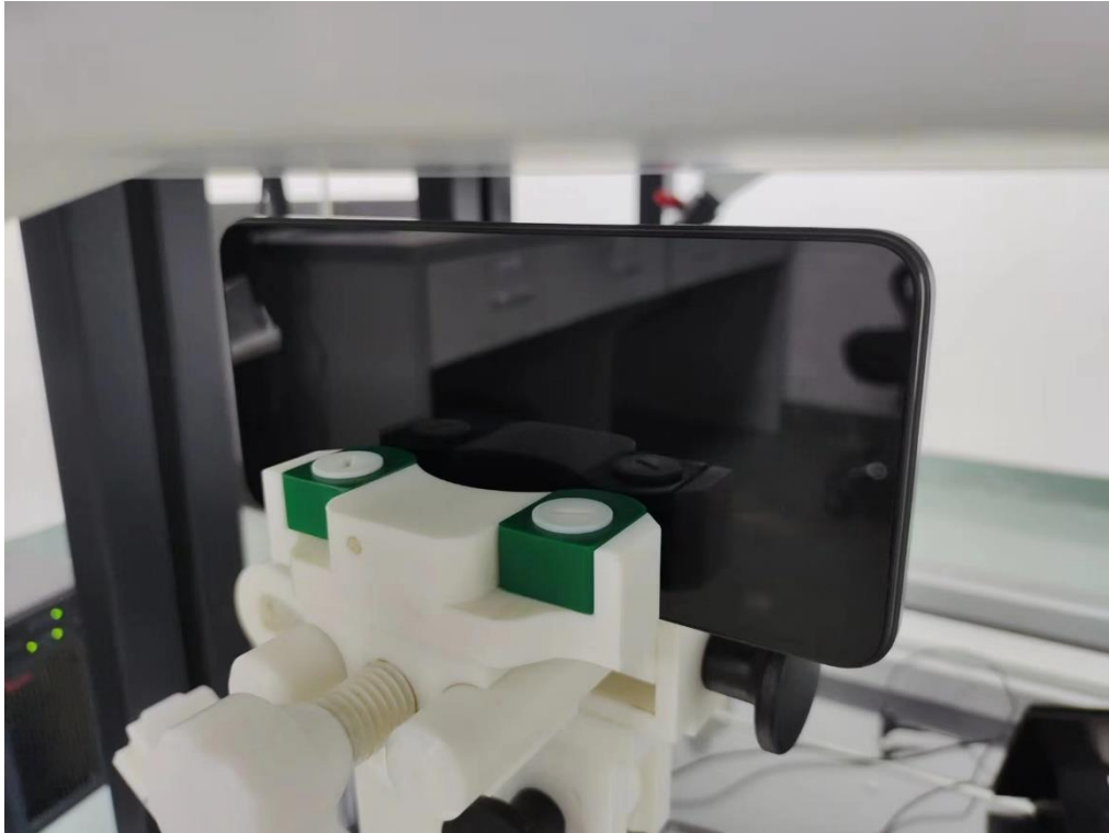
Body Left side (separation distance is 10mm)
