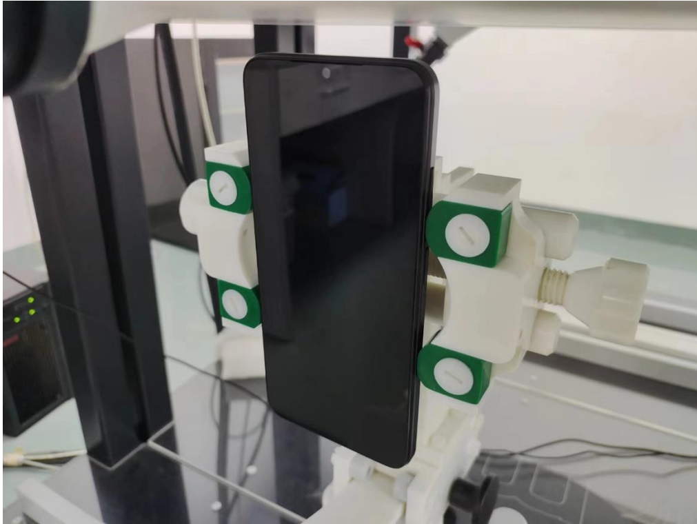
Body Top side (separation distance is 10mm)
