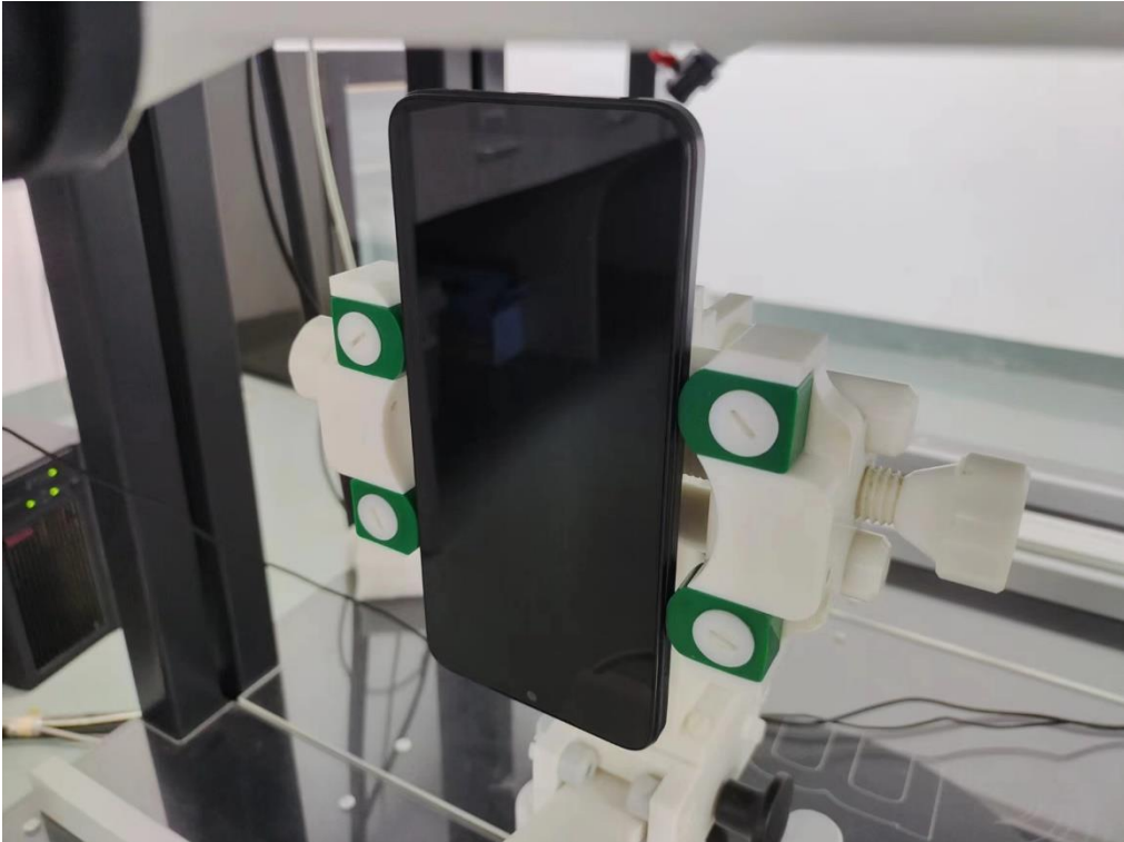
Body Bottom side (separation distance is 10mm)
