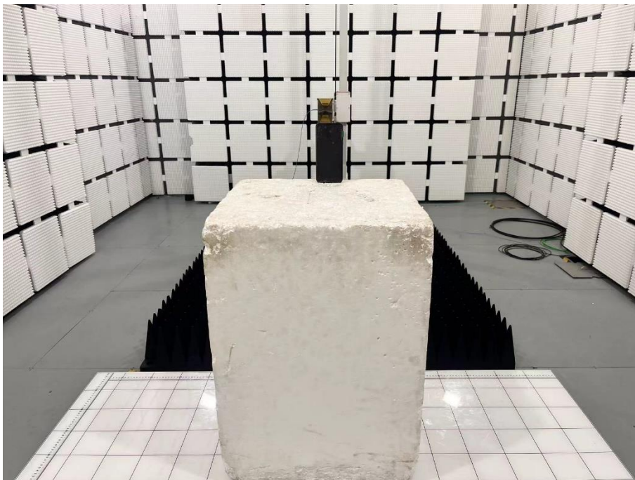
Set-up for Radiated Spurious Emission, Above 1GHz
