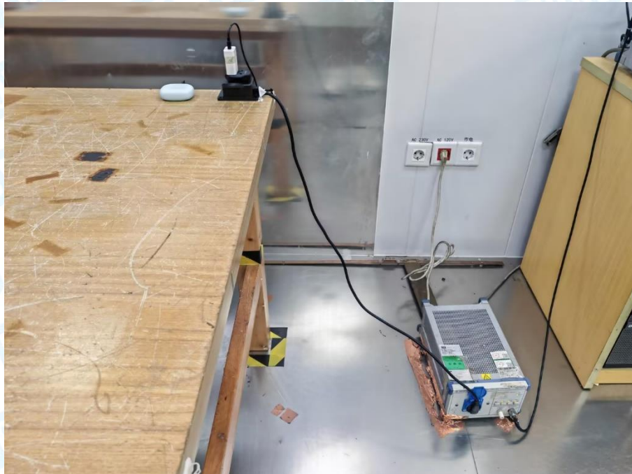
Photo of Setup for Radiated Emission (30MHz~1GHz)
