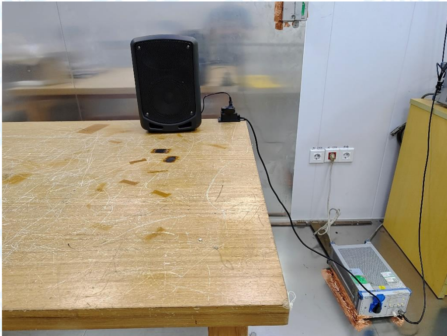
Photo of Setup for Radiated Emission (30MHz~1GHz)
