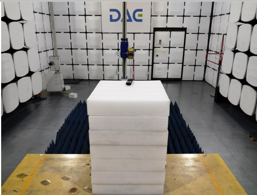
Emissions in frequency bands (above 1GHz)
