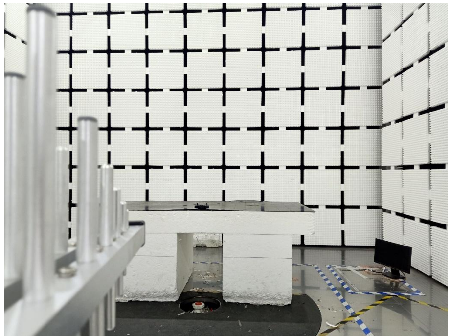
Radiation Emission Test Setup (30MHz to 1GHz)
