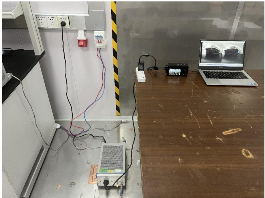
Conducted Emission Test Setup
