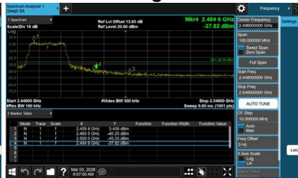
CH01 – 10th Harmonic of the fundamental frequency
