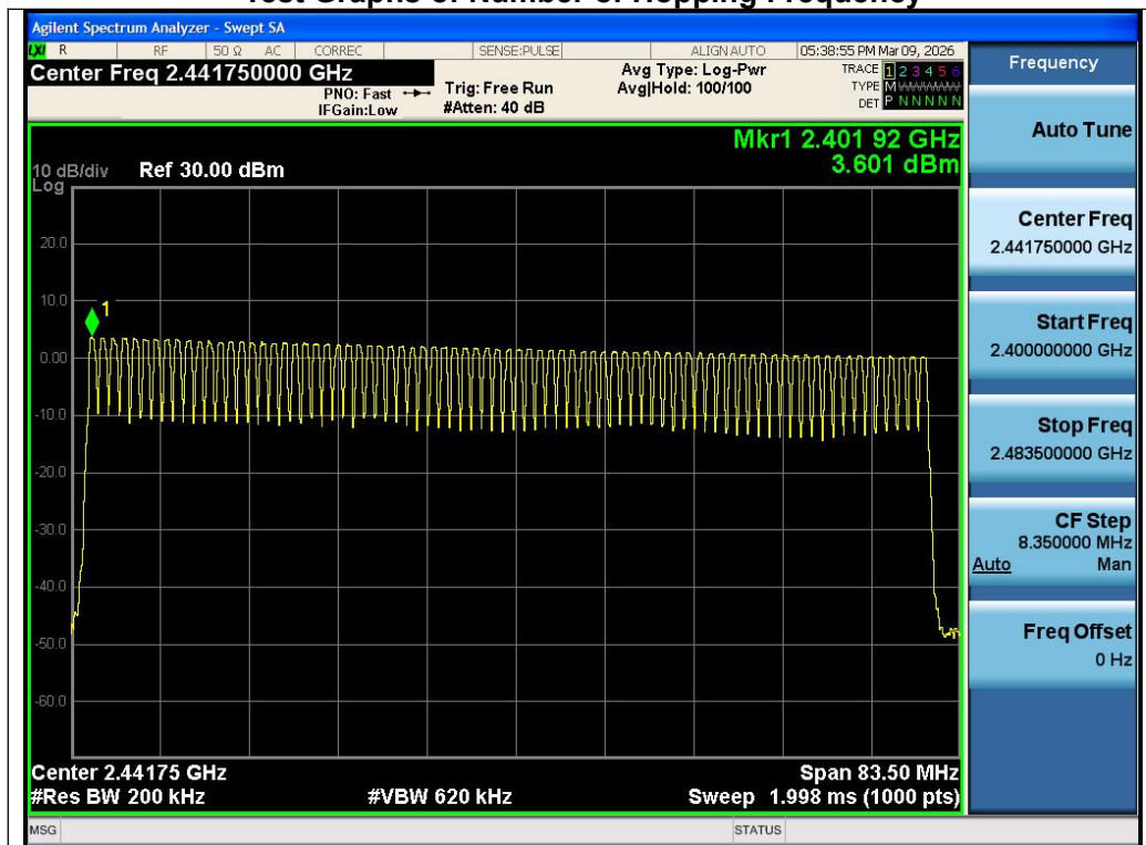
Test_Graph_BR_HOP_ANT1_NA_1Mbps_Number of Hopping
