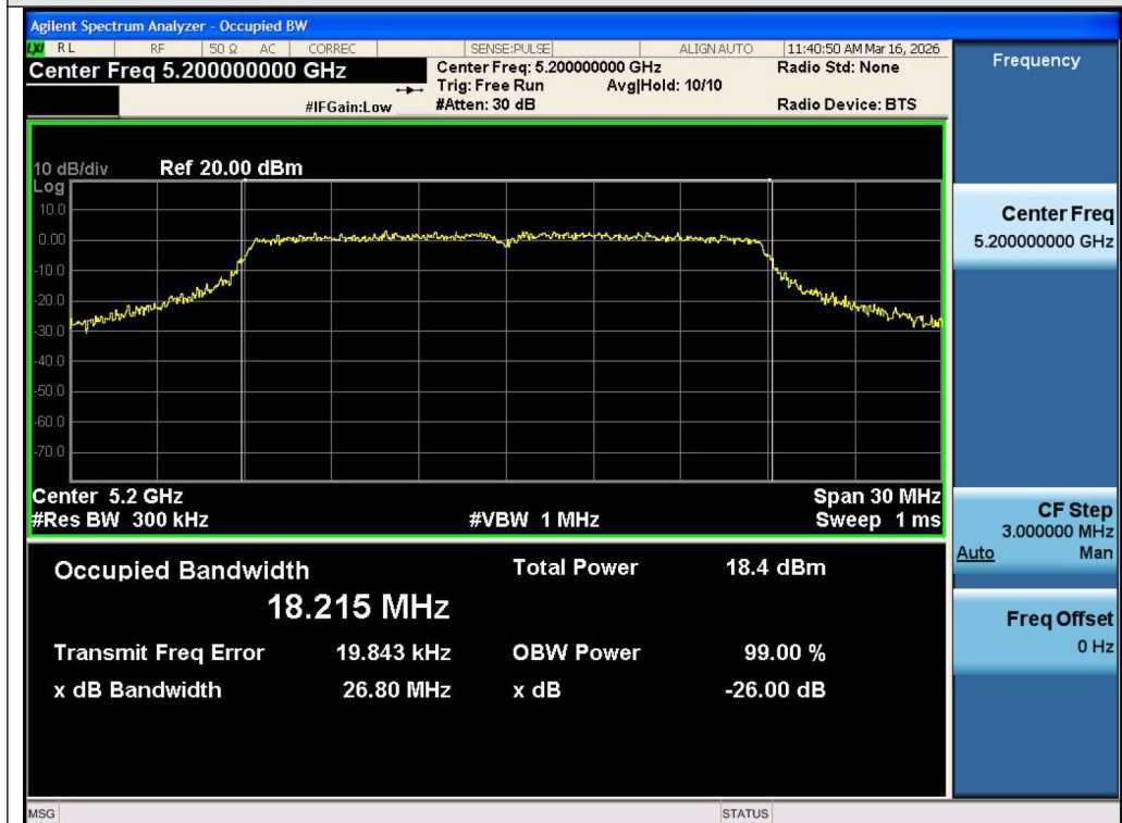
Test_Graph_802.11ac20_ANT1_5200_MCS0_OBW
