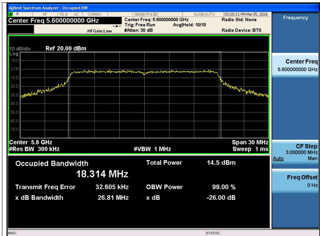
Test_Graph_802.11n20_ANT1_5600_MCS0_OBW
