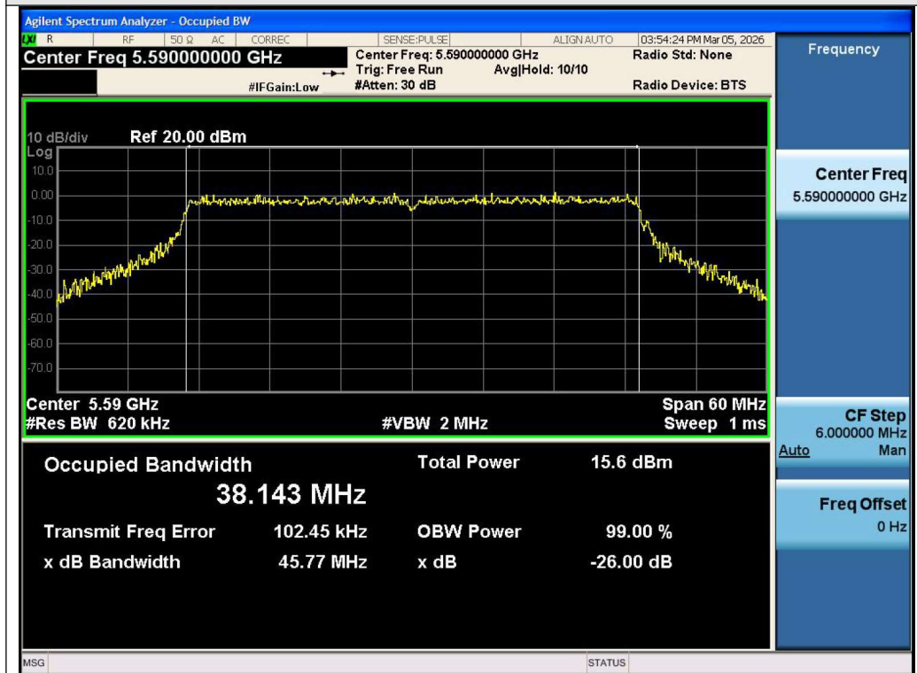
Test_Graph_802.11ax40_ANT1_5590_MCS0_OBW
