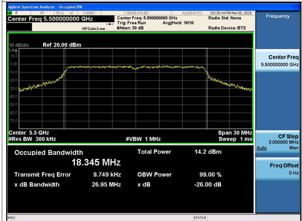
Test_Graph_802.11ac20_ANT1_5500_MCS0_OBW
