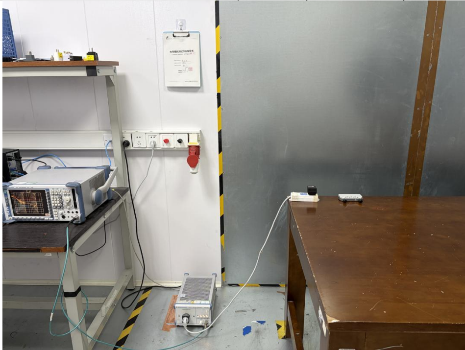
Conducted emissions at AC power line (150kHz-30MHz)
