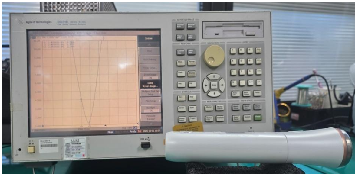
Figure 4.2.1 Test by network analyzer
