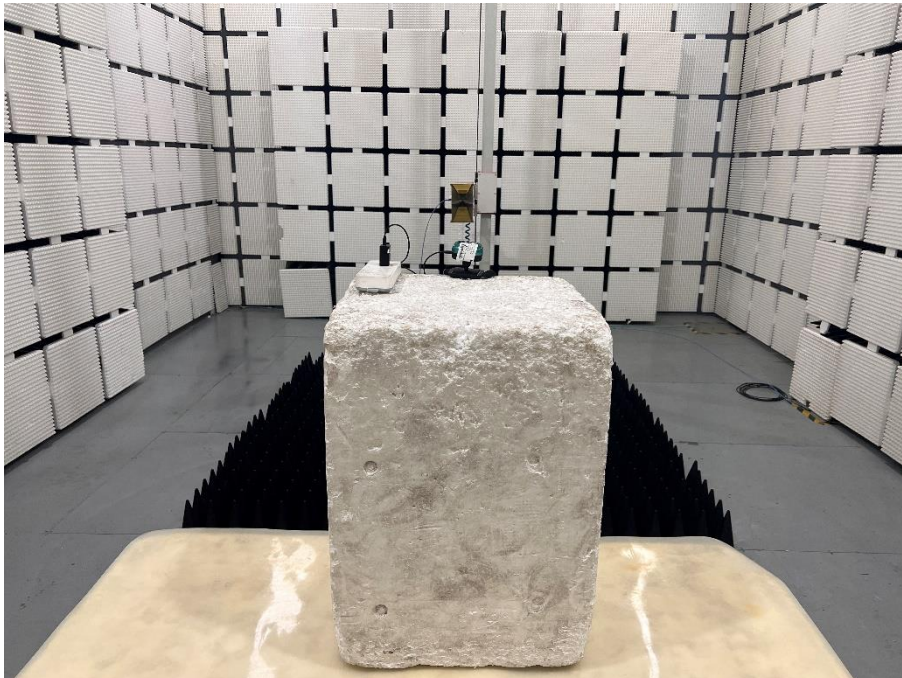
Set-up for Radiated Spurious Emission, Above 1GHz
