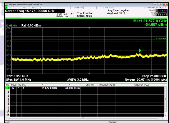
Spurious Emission:5350~25000.0 MHz IEEE 802.11ac_Channel 38_40MHz_Antenna 0
