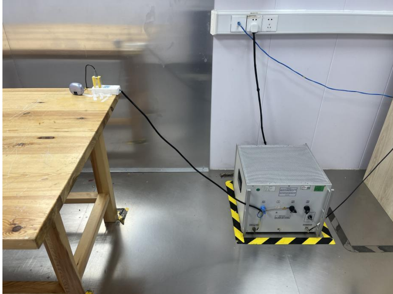
Radiated Emissions From 30M-1GHz
