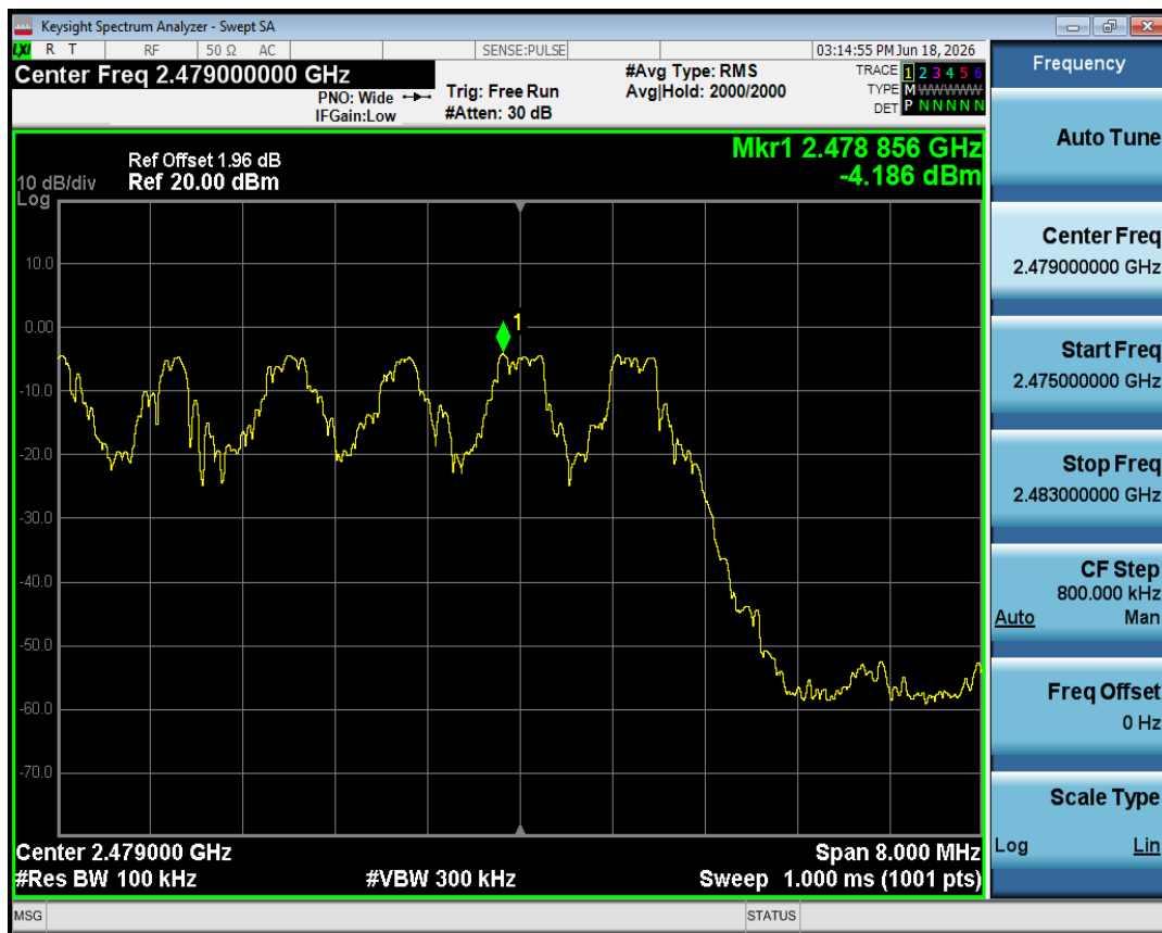
Band Edge(Hopping) NVNT GFSK 2479MHz ANT_L Hopping Ref
