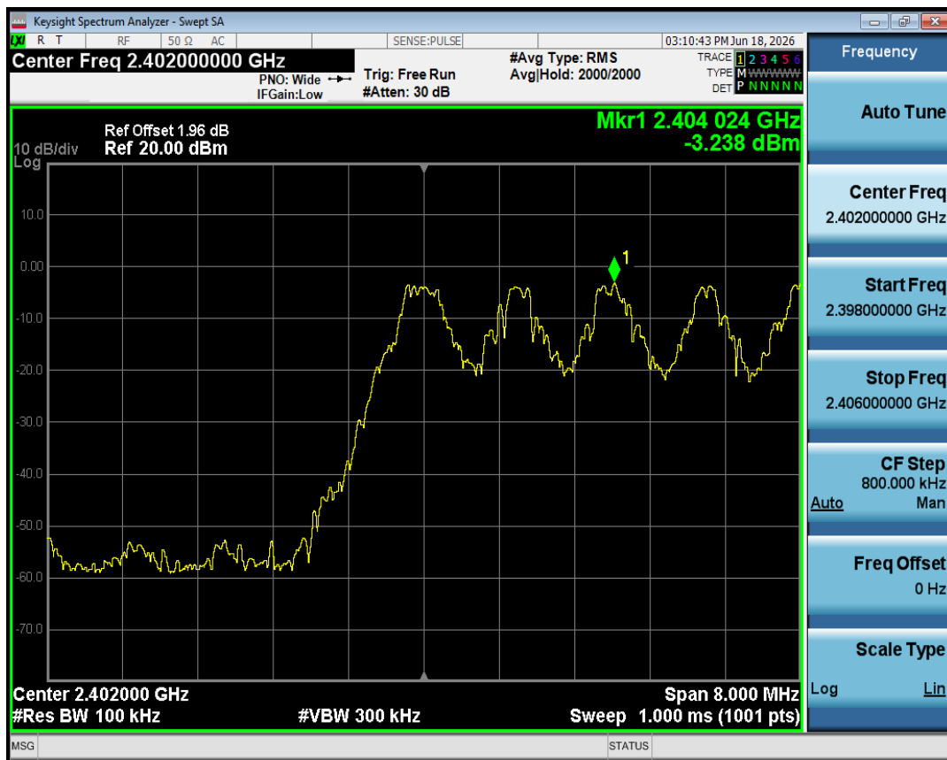
Band Edge(Hopping) NVNT GFSK 2402MHz ANT_L Hopping Ref
