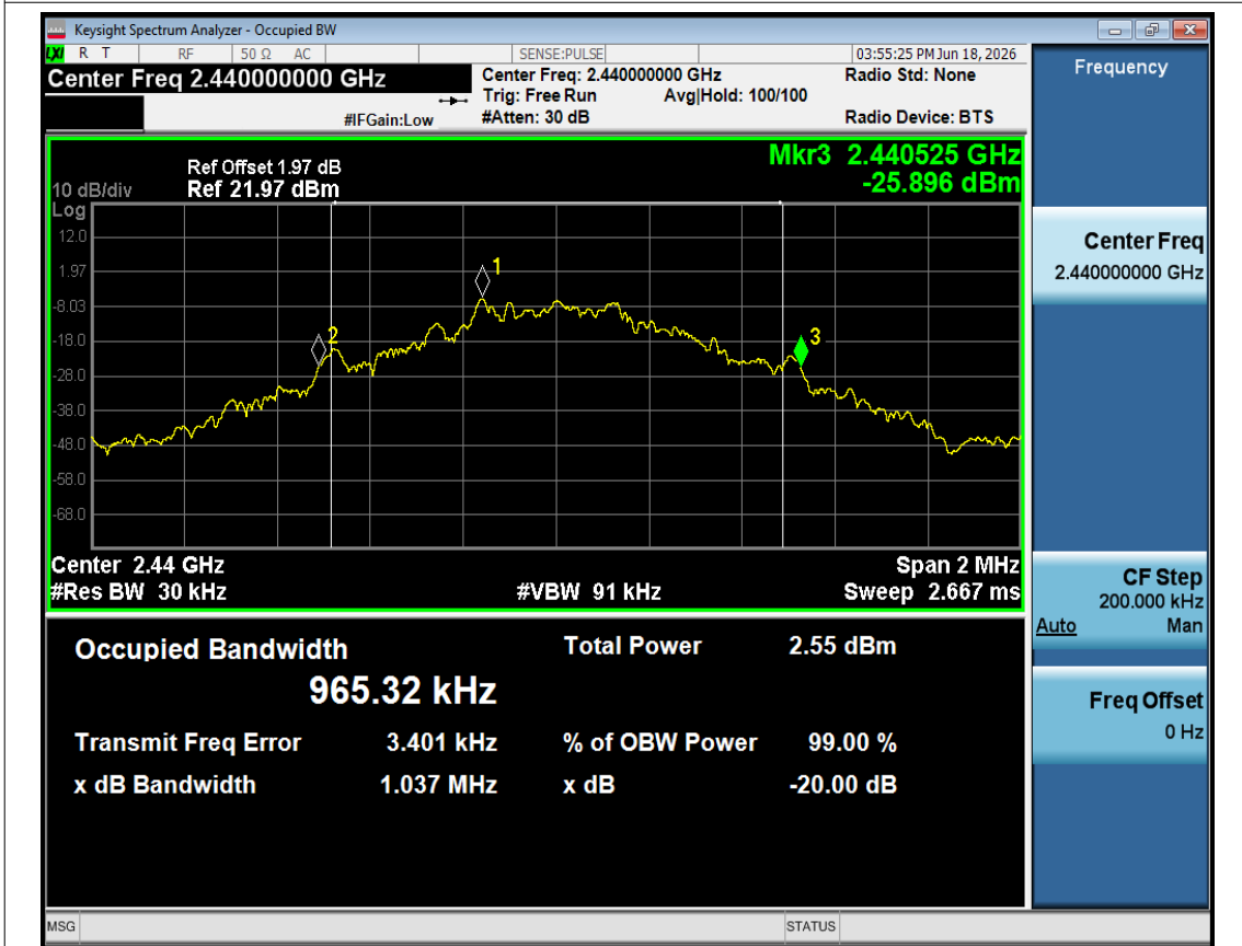
-20dB Bandwidth NVNT GFSK 2440MHz ANT_L
