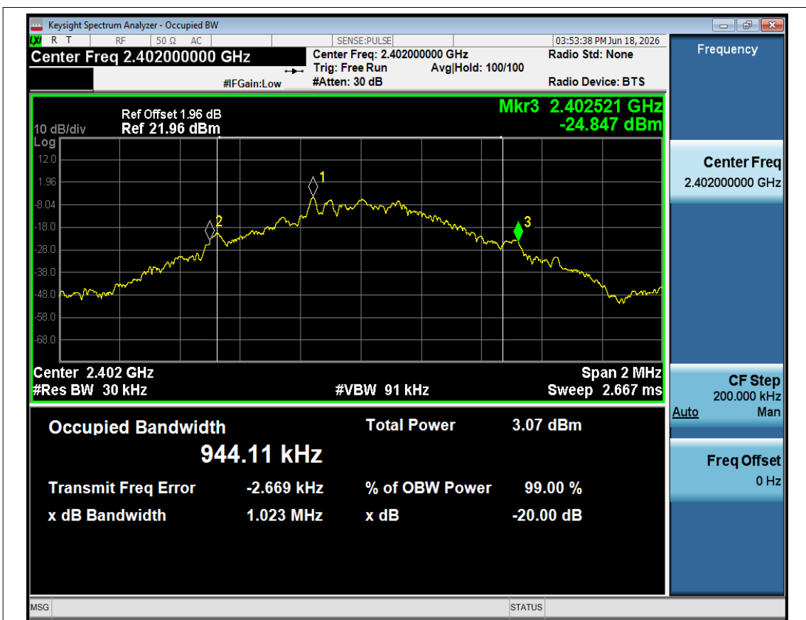
-20dB Bandwidth NVNT GFSK 2402MHz ANT_L
